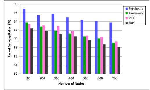
Fig. 7: Packet delivery ratio in WSN # 2
