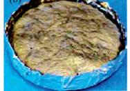
**Figure 11.** (a) Effect of various nanofillers on mass loss rate when PMMA composites are subjected to an external radiant flux of 50 kW  $m^{-2}$  in nitrogen. (b) Residue from the 0.5 wt % SWNT/PMMA composite after the gasification test showing a free-standing nanotube structure. Reprinted with permission from ref 111.
