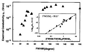
**Figure 8.** Electrical conductivity of a 2 wt % SWNT/PMMA composite along the alignment direction with increasing nanotube isotropy. Nanotube alignment is assessed using X-ray scattering where fwhm = 0 is perfectly aligned and fwhm = 180 is isotropic. Inset: a log-log plot of electrical conductivity vs reduced fwhm determines the critical alignment, fwhm<sub>c</sub>. Reprinted with permission from ref 23. Copyright 2005 American Physical Society.
