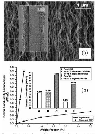
**Figure 10.** (a) SEM image of the side view of an aligned MWNT array. Inset: a high-resolution TEM image of an isolated MWNT showing eight nested nanotubes. (b) Thermal conductivity enhancement ( $\kappa_{composite} - \kappa_{matrix}$ ) vs weight fraction of MWNT in both aligned and unaligned nanocomposites. Inset: thermal conductivity for selected MWNT/silicone elastomer composites. Reprinted with permission from ref 64. Copyright 2005 Wiley-VCH.
