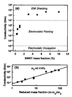
**Figure 7.** (a) Electrical conductivity of SWNT/polycarbonate nanocomposites as a function of nanotube loading, showing a typical percolation behavior. Dashed lines represent the lower limits of electrical conductivity required for the specified applications. (b) Electrical conductivity as a function of reduced mass fraction of nanotubes, showing a threshold of 0.11 wt %. Reprinted with permission from ref 89. Copyright 2003 American Institute of Physics.
