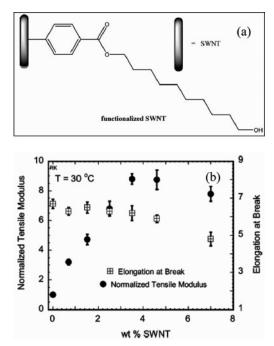
**Figure 6.** (a) Structure of the functionalized SWNT used for the fabrication of PDMS nanocomposite (SWNT not drawn to scale). (b) Composition dependence of the normalized tensile modulus ( $E_{\text{composite}}/E_{\text{PDMS}}$ ) and the elongation at break ( $L_{\text{break}}/L_{\text{initial}}$ ) for SWNT/PDMS nanocomposites. From ref 17.
