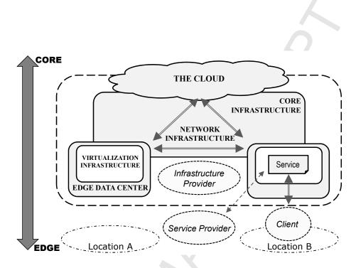
Figure 1: Functional structure of edge paradigms
