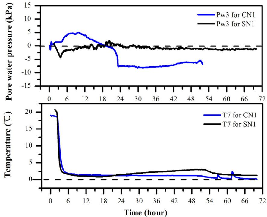
Fig. 5. Variations of pore water pressure in the unfrozen zone of the sandy soil sample SN1 and the silty clay sample CN1.
