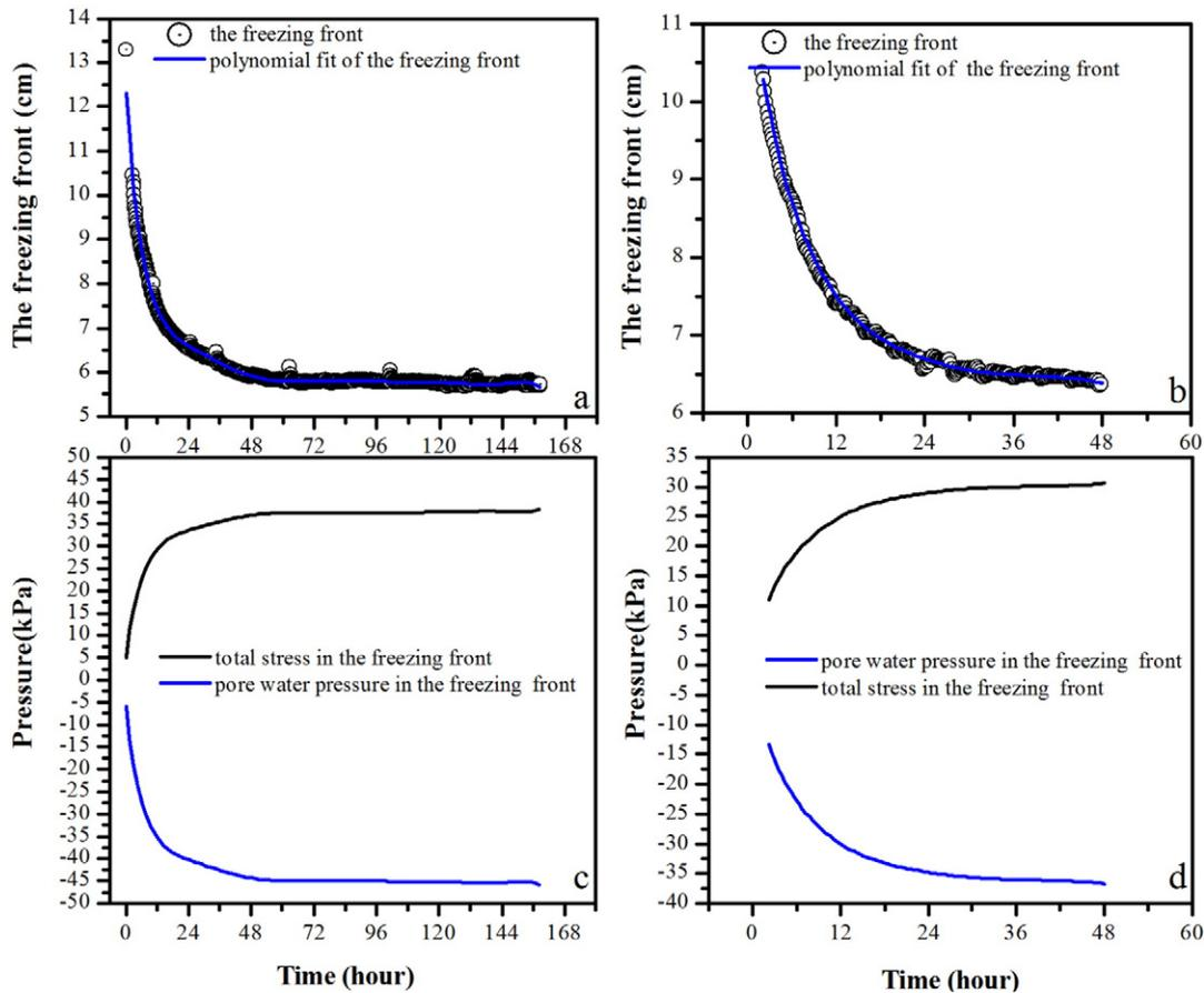
Fig. 10. The boundary conditions in the freezing front, including the (a) evolution of the freezing front during experiment CN2, (b) evolution of the freezing front during experiment CN1, (c) total stress and pore water pressure at the freezing front with time during experiment CN2, and (d) the total stress and pore water pressure in the freezing front with time during experiment CN1.
