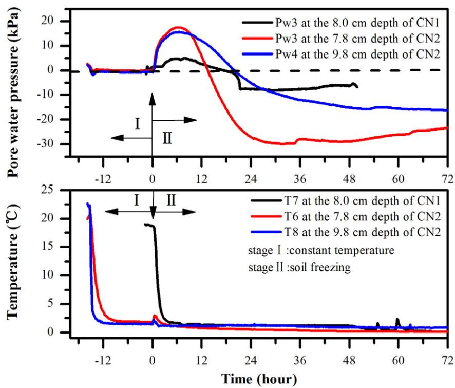
Fig. 4. Variations of the pore water pressure in the unfrozen zone of silty clay soil samples with different water supply conditions, soil sample CN1 with an open-system condition and CN2 with a closed-system condition.
