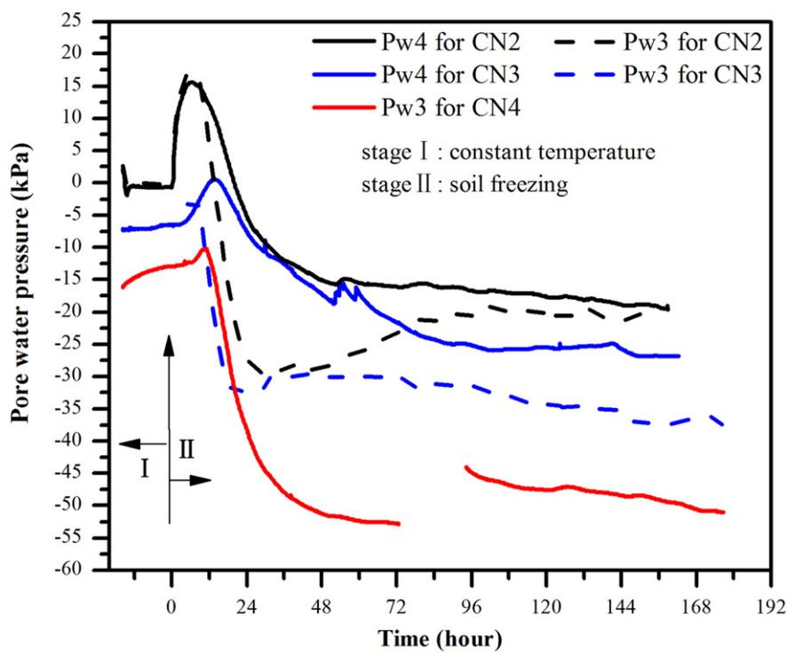
Fig. 6. Pore water pressure variations in the unfrozen zone with different initial moisture contents.
