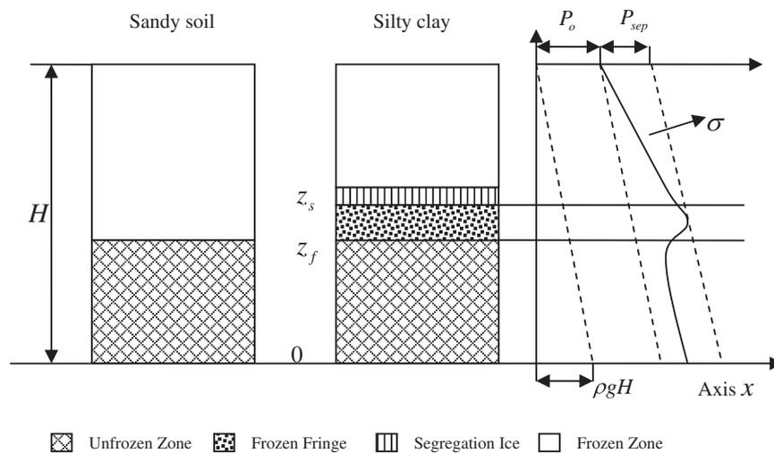
Fig. 8. Sketch of the zones and total stress during freezing of sandy soil and silty clay samples.
