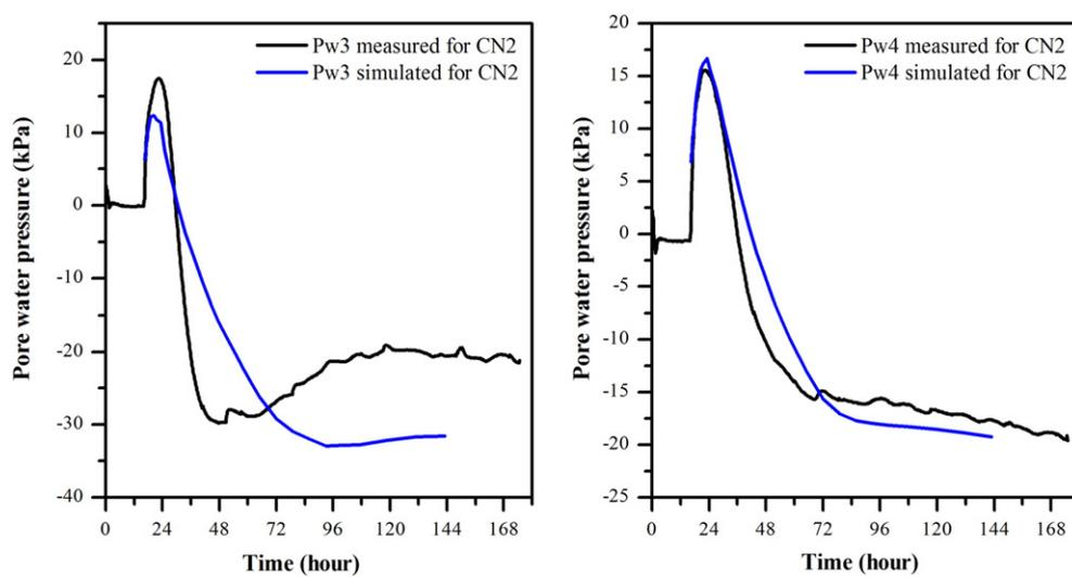
Fig. 11. Comparison of the measured and simulated pore water pressures in the unfrozen zone during closed-system freezing of CN2.
