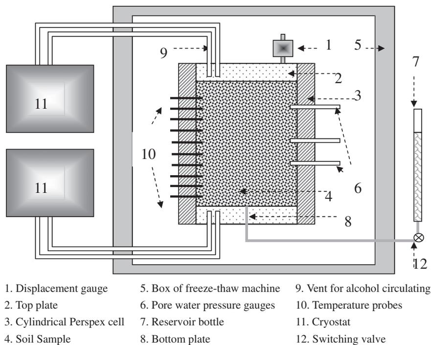
Fig. 1. Sketch of the freeze-thaw testing system.
