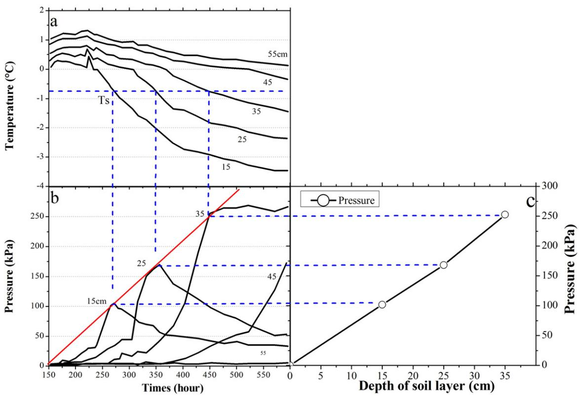
**Fig. 9.** Evolution of stress during freezing. (a) Variations of temperature over time at different depths, (b) variations of frost heaving stress over time at different depths, and (c) the dependency of the frost heaving stress on the soil layer depth.
