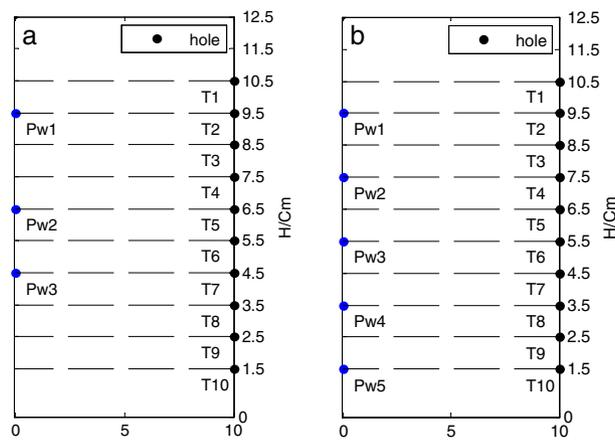
Fig. 2. Hole arrangements of two similar cylindrical Perspex cells.
