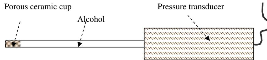
Fig. 3. Sketch of the pore water pressure probe.
