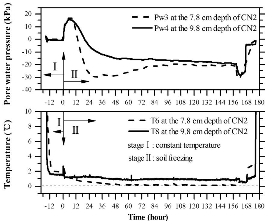
Fig. 7. Pore water pressure variations at different depths during the freezing of the CN2 sample.
