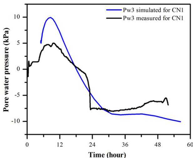
Fig. 12. Comparison of the measured and simulated pore water pressures in the unfrozen zone during open-system freezing of CN1.
