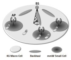
Fig. 3. System architecture proposed for 5G.
