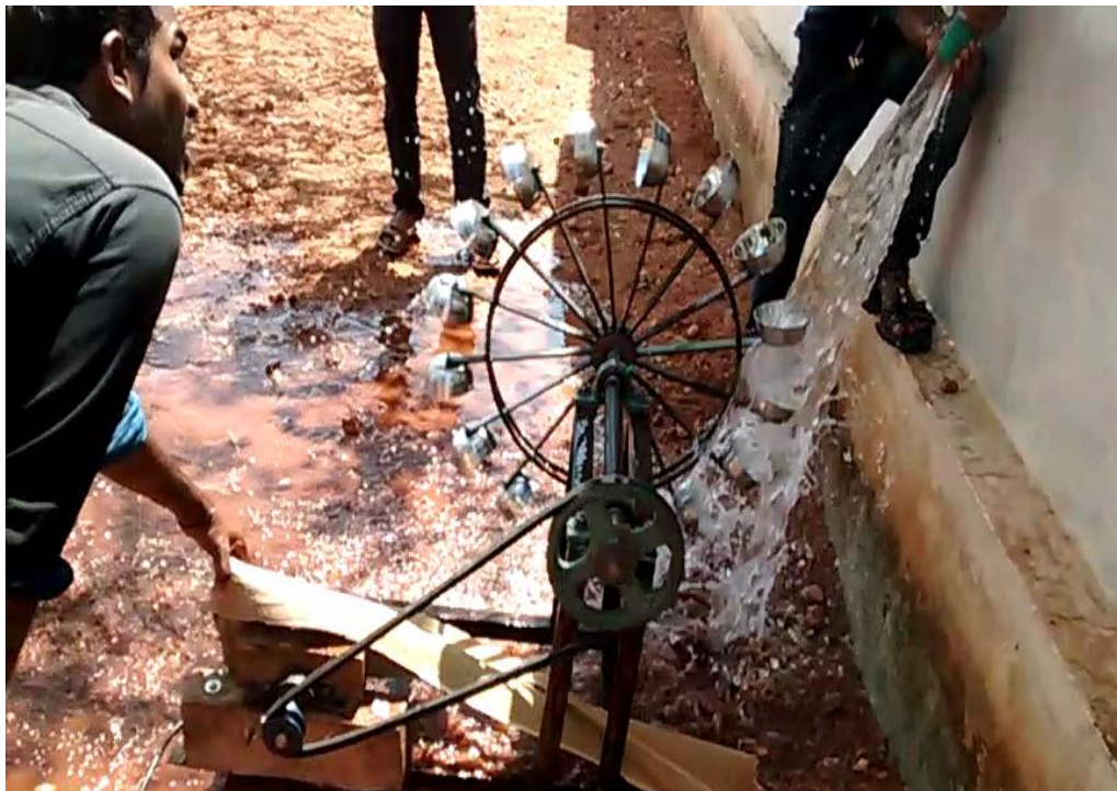
Fig1: Pelton Water Wheel.
