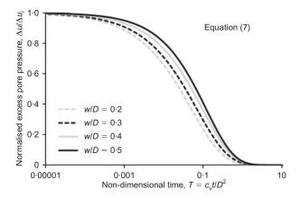
Fig. 6. Fitted invert pore pressure dissipation-time histories for range of embedment
