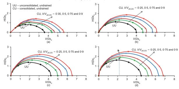
Fig. 9. Failure envelopes for unconsolidated and consolidated breakout: (a) w/D = 0.2; (b) w/D = 0.3; (c) w/D = 0.4; (d) w/D = 0.5
