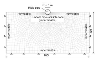
Fig. 1. Finite-element model (w/D = 0.5)
