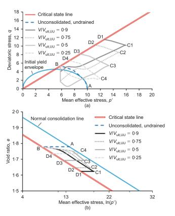
Fig. 7. Stress paths at pipe invert during loading and consolidation (w/D = 0.5): (a) p'-q space; (b)  $e-\ln(p')$  space
