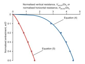
Fig. 3. Variation of unconsolidated, undrained, vertical and horizontal capacity with initial embedment
