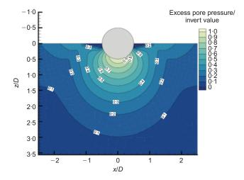
Fig. 4. Distribution of excess pore-water pressure after undrained penetration
