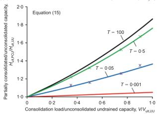
Fig. 14. Effect of partial consolidation on undrained horizontal capacity (w/D = 0.2)
