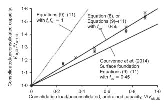
Fig. 10. Gain in undrained vertical capacity due to consolidation
