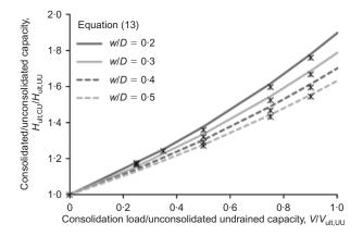
Fig. 11. Gain in undrained horizontal capacity due to consolidation
