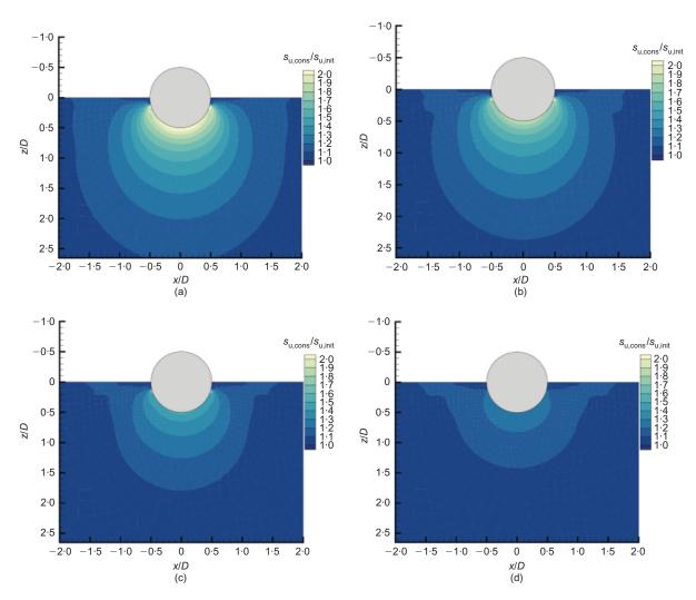
Fig. 8. Distribution of shear strength enhancement due to consolidation: (a)  $V/V_{\rm ult,UU}=0.9$ ; (b)  $V/V_{\rm ult,UU}=0.75$ ; (c)  $V/V_{\rm ult,UU}=0.5$ ; (d)  $V/V_{\rm ult,UU}=0.25$
