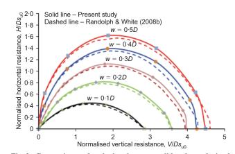
Fig. 2. Comparison of calculated, unconsolidated, undrained, pipe breakout resistance and theoretical solution
