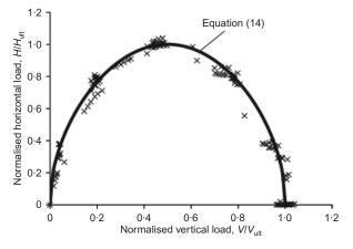
Fig. 12. Normalised failure envelopes for consolidated, undrained breakout
