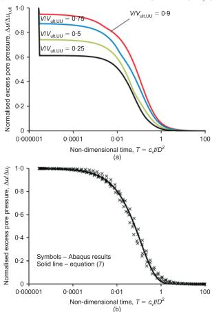
Fig. 5. Invert pore pressure dissipation—time histories during consolidation (w/D=0.5): (a) normalised by initial excess pore pressure at vertical capacity  $(\Delta u_{i,ult})$ ; (b) normalised by initial excess pore pressure under operative consolidation load  $(\Delta u_i)$
