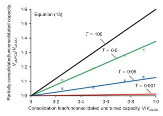
Fig. 13. Effect of partial consolidation on undrained vertical capacity
