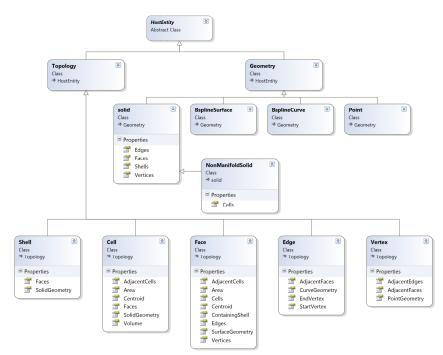
Figure 4: The DesignScript geometry and topology classes, with their properties
