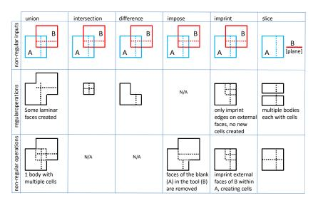
Figure 3: The result of regular or non-regular Boolean operations with non-manifold inputs
