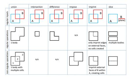
Figure 2: The result of different regular or non-regular operations with manifold inputs. Note: some operations (union and intersection) are symmetric, while other operations (difference, impose) are asymmetric. With asymmetric operation there is the convention that one input is referred to as the 'part' (A), the other input is referred to as the 'tool' (B). We can compare:
