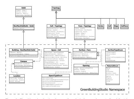
Figure 8: Class hierarchy showing the use of topological super classes (cell and face) in relation to the sub classes (space and surface) within the Green Bulding studio namespace.
