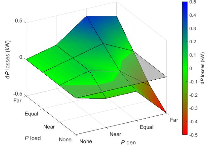
Figure 7. Difference of cumulative losses on the MV/LV transformer and LV network between  $Q_{\text{GEN}} = 0$  and  $Q_{\text{GEN}} = f(P_{\text{GEN}}, U)$  reactive power regulation in LV network with cable lines
