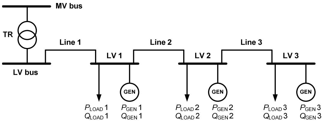
Figure 2. Network model for simulations
