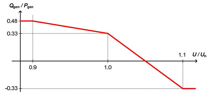
Figure 1. Proposed optimized reactive power characteristic
