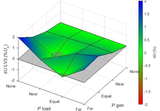
Figure 4. Difference of relative voltage changes at node LV3 between  $Q_{GEN} = 0$  and  $Q_{GEN} = f(P_{GEN}, U)$  reactive power regulation regarding the desired voltage in LV network with overhead lines
