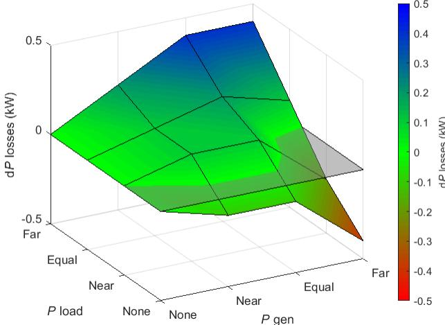
Figure 6. Difference of cumulative losses on the MV/LV transformer and LV network between  $Q_{\text{GEN}} = 0$  and  $Q_{\text{GEN}} = f(P_{\text{GEN}}, U)$  reactive power regulation in LV network with overhead lines
