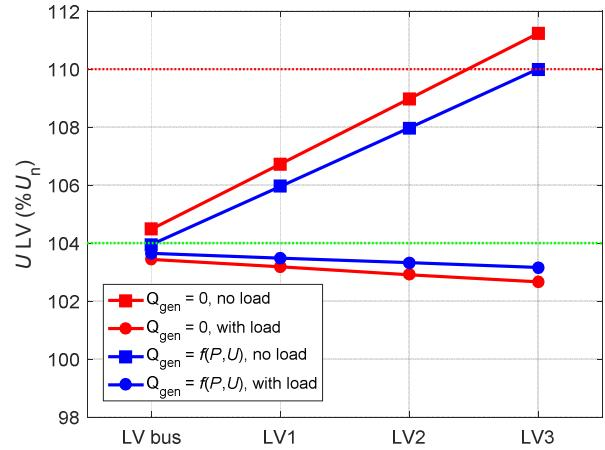
Figure 3. Effect of different reactive power regulations on the voltage profile in the LV cable network
