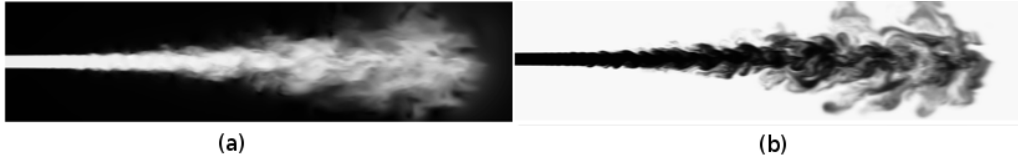
Figure 7: Instantaneous results of the nitrogen injector. (a) velocity magnitude ( 0 \leq |\mathbf{u}| \leq 5.6 \text{ m/s} ); (b) temperature ( 125.6 \leq T \leq 306.7 \text{ K} )
