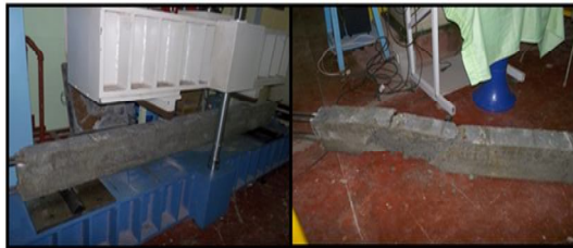
Figure 3.7 Conventional Beam Tested in RFTM
