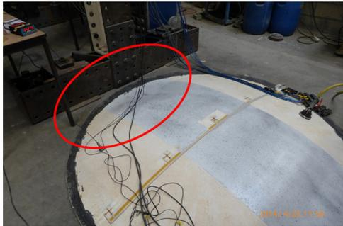
Fig. 7. The shell buckles locally near the edge.
