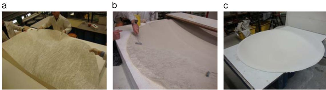
**Fig. 4.** The GFTR-IPC dome is produced in layers. (a) First, the fibre mats are placed in the foam mould. (b) Second, the mats are impregnated with the matrix IPC. (c) After hardening, the dome is inverted and a thin GFTR-IPC shell is obtained.
