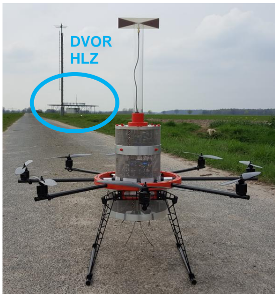
Figure 9: Reference measurement on ground close to DVOR HLZ
