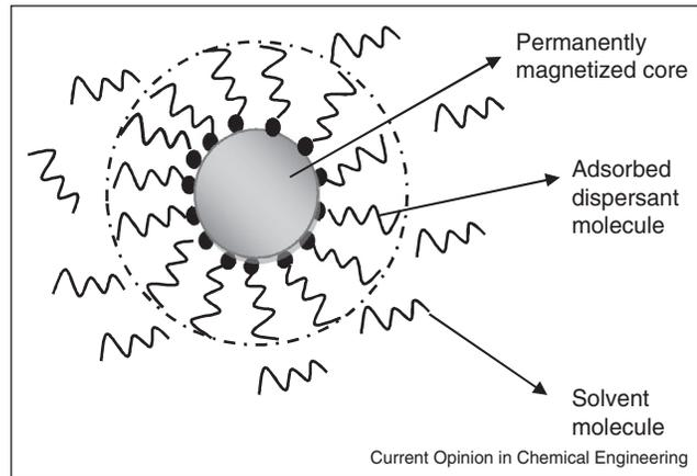
Adsorption of the long chain molecules onto the particle surface provides steric repulsion increasing the hydrodynamic radius [27].
