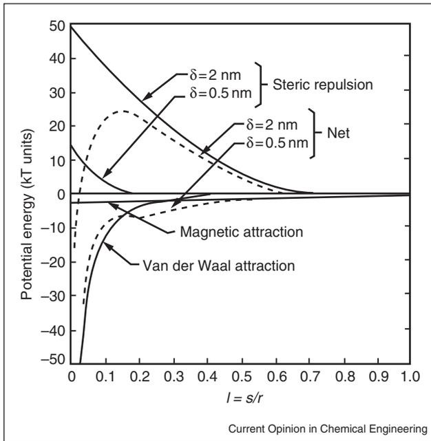
Illustration of magnetic attractive energy, van der Waals attractive energy and steric repulsion energy and the net potential energy for different lengths of adsorbed molecule,  $\delta$ . The ratio between the interparticle distance and the radius of the particle is denoted as ' $l = s/r$ ' [27].
