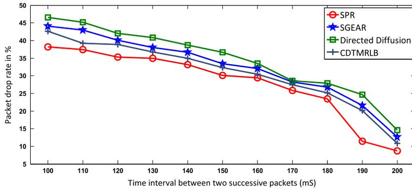
Fig. 8. Average packet drop rate at decreasing traffic load.
