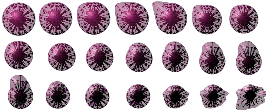
Figure 3. Variable forms of ROBOBBLE can be created through the use of 24 linear actuators.
