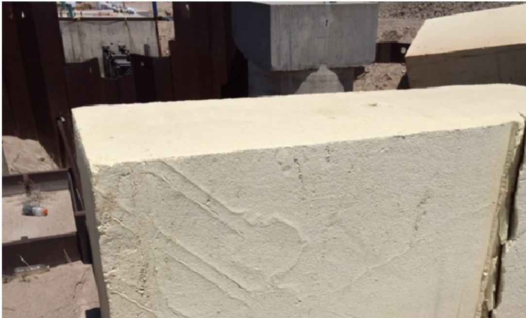
Figure 3. Photograph of the compressed geofoam along with shear plane that developed at the edge of the pile cap.
