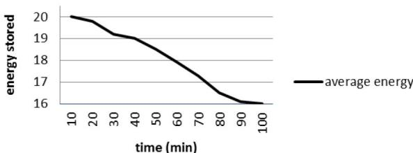
Fig. 3. Average Energy Stored at nodes vs. Time
