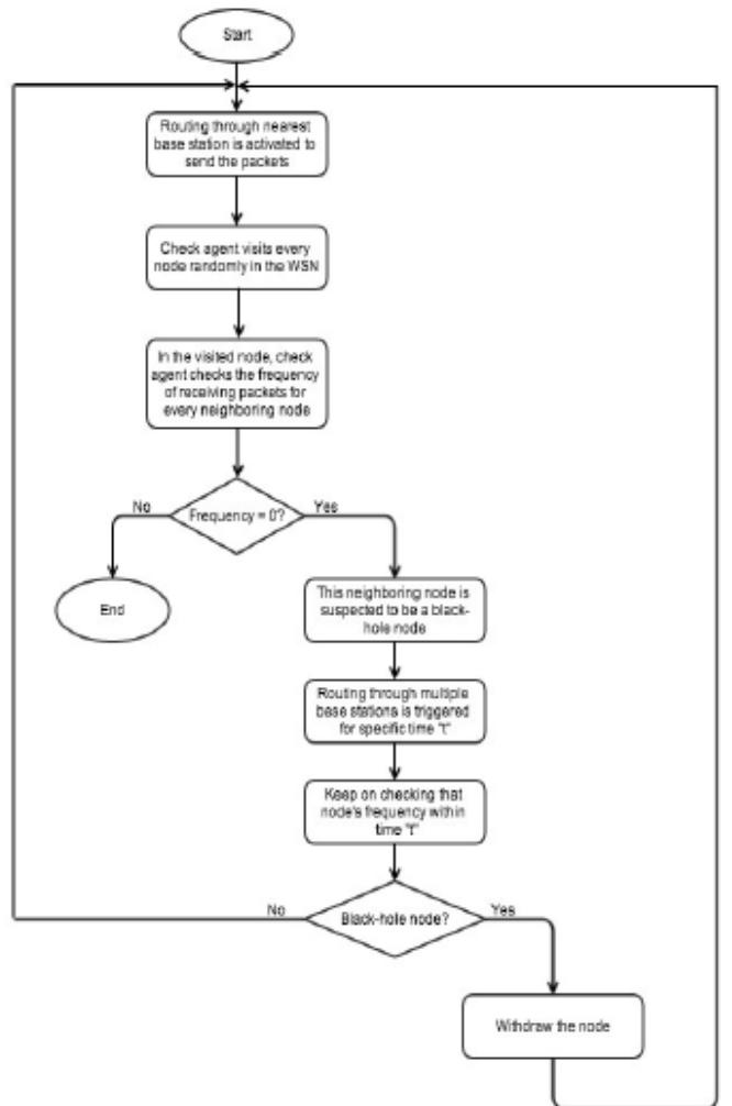
Fig. 2. Detection Process Steps
