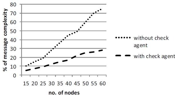
Fig. 5. Message Complexity vs. No. of Nodes
