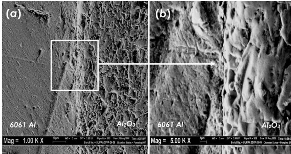
Fig. 4. Interface of specimen welded observed under FESEM at 1250 rpm (a) 1000× and (b) 5000×.
