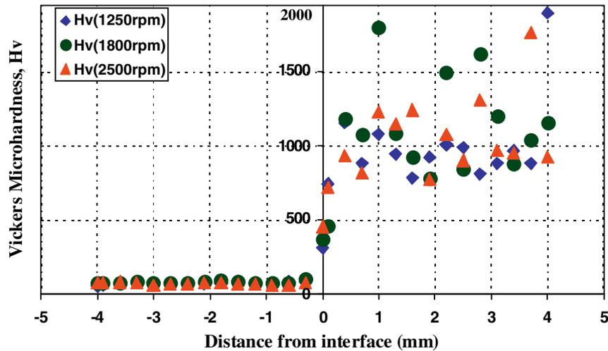
Fig. 10. Microhardness traverse of 6061 Al alloy-alumina friction welded joints.
