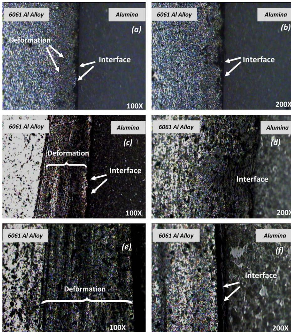
**Fig. 3.** Optical images of interface properties of specimens welded at (a, b) 1250 rpm, (c, d) 1800 rpm, (e, f) 2500 rpm magnification 100 $\times$ , 200 $\times$ .
