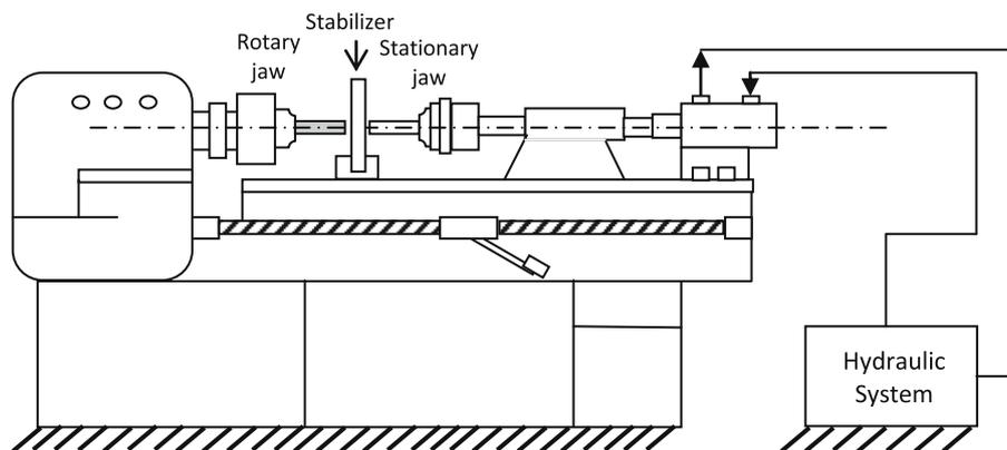
Fig. 1. A set up of a Friction Welding Machine.
