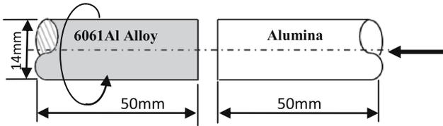
**Fig. 2.** Shapes and dimensions of specimens used for friction welding.
