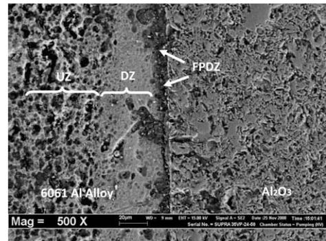
Fig. 7. Interface of specimen welded observed under FESEM at 1800 rpm after etching in 1%NaOH. Time = 15 min.
