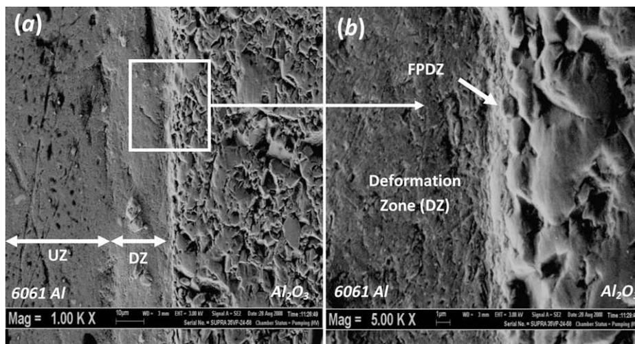
Fig. 6. Interface of specimen welded observed under FESEM at 1800 rpm (a) 1000× and (b) 5000×.
