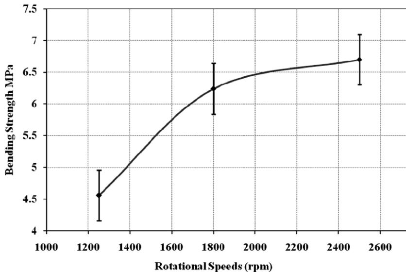
Fig. 11. Four point bending strength of 6061 Al alloy-alumina friction welded joints.
