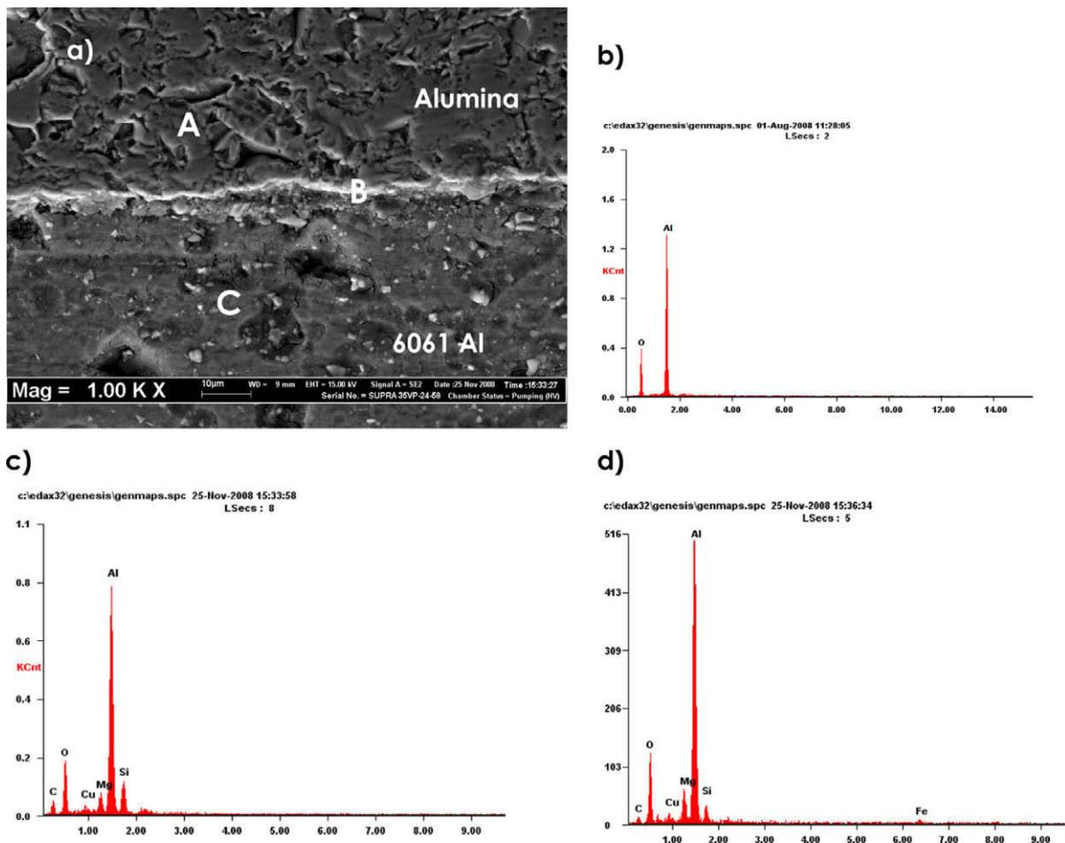
Fig. 9. (a) Micrograph of joining compound, (b) EDX analysis at A, (c) EDX analysis at B and (d) EDX analysis at C.
