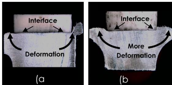
Fig. 5. Shapes of Burrs in the joining between alumina-6061 Al alloy (a) 1250 rpm and (b) 2500 rpm.
