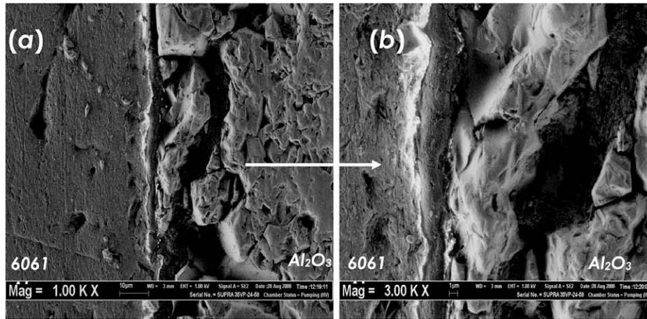
Fig. 8. Interface of specimen welded observed under FESEM at 2500 rpm (a) 1000 $\times$  and (b) 3000 $\times$ .
