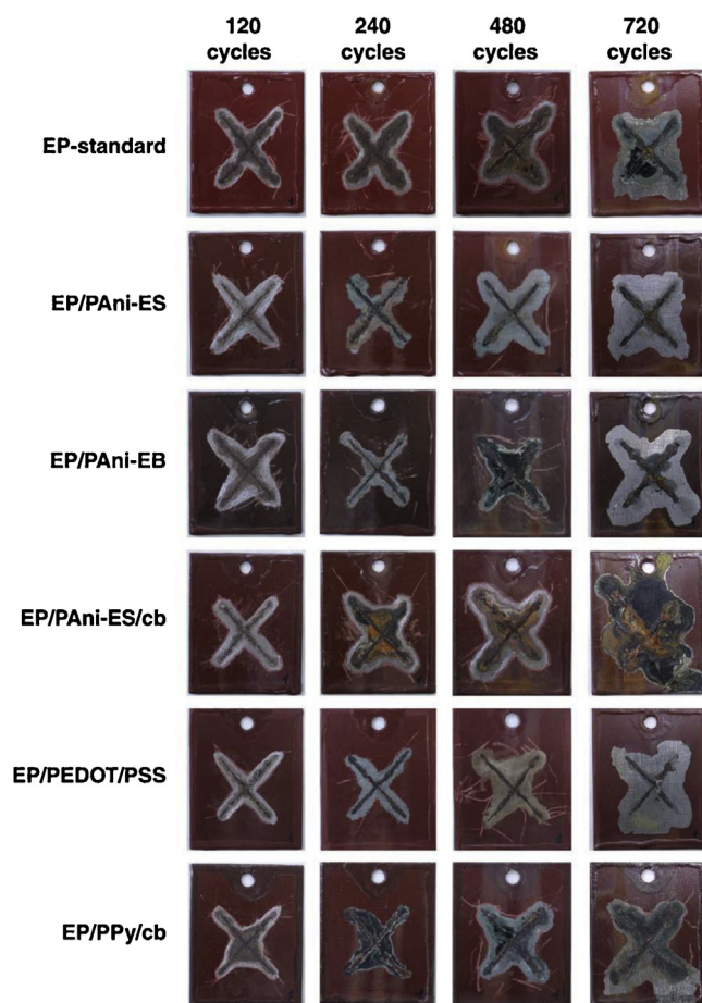
Fig. 6. Scrapped test panels of EP-standard, EP/PAni-ES, EP/PAni-EB, EP/PAni-ES/cb, EP/PEDOT/PSS and EP/PPy/cb after 120, 240, 480 and 720 corrosion cycles. Corrosion resistance was evaluated according to the ASTM D-1654.
