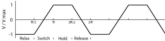
Fig. 3. Four-phased signal for clocking (adiabatic switching).
