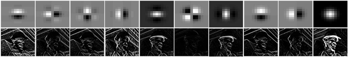
Fig. 4. Basis filters of H_2 and their responses. Top row: a temporal slice of each of the ten 3D basis filters at t = 6 . Bottom row: the corresponding temporal slice of the 3D outputs for ten frames of the Foreman sequence.
