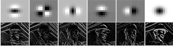
Fig. 3. Basis filters of G_2 and their responses. Top row: a temporal slice of each of the six basis filter at t = 6 . Bottom row: the corresponding temporal slice of the 3D outputs for ten frames of the Foreman sequence.
