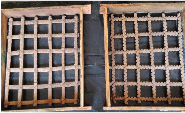
Fig. 6. Casting of PTBRC and GTBRC slab panels.
