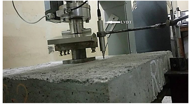
Fig. 9. Slab panel subjected to central concentrated load.
