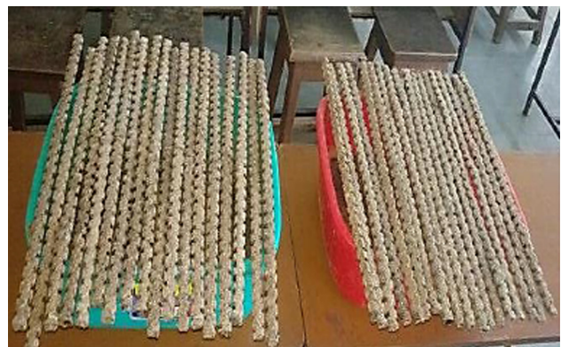
Fig. 3. Preparation of grooved bamboo reinforcement.
