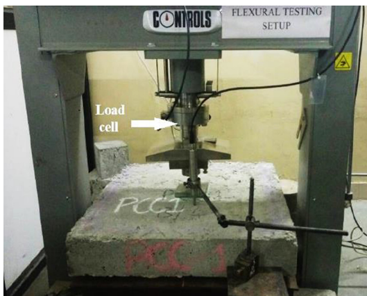
Fig. 8. FTM used during slab testing.
