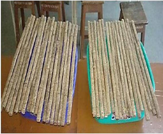
Fig. 4. Preparation of plain bamboo reinforcement.
