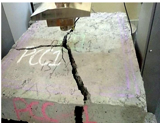
Fig. 11. Crack pattern in PCC slab.
