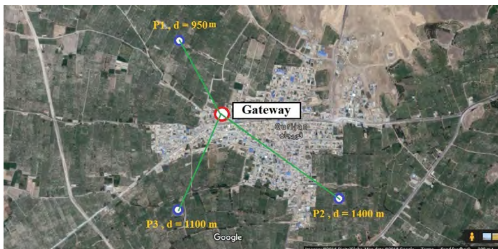
Fig. 9. Network layout of a WSN system used in the vineyards. P1, P2, and P3 represent Yovşanlıq, Minə, and Mıncıqlı vineyards, respectively.
