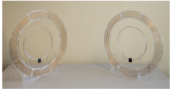
Fig. 5. Photograph of the transmitter and receiver used in wireless power system. Outside diameter of the large coils is 59 cm.
