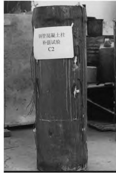
(b) Dilation of steel tube
