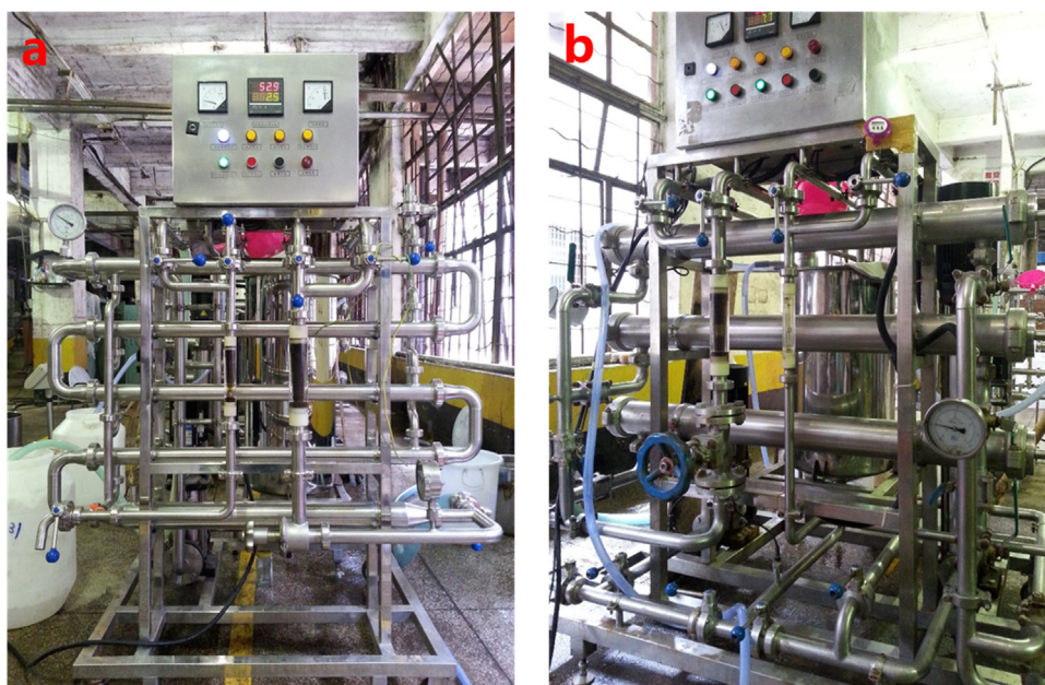
Fig. 2. Photographs of the pilot equipment for (a) tubular loose UF module (clarification of raw sugarcane juice) and (b) spiral wound tight UF and NF modules (decolorization and concentration of sugarcane juice).
