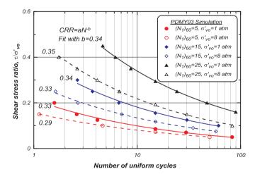
Fig. 11. Cyclic shear stress ratio versus number of uniform loading cycles in undrained DSS simulations to trigger liquefaction defined as single-amplitude shear strain of 3% (no static shear stress  $\alpha = 0$ ).
