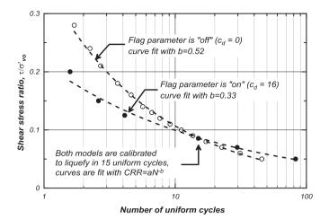
Fig. 5. Effects of input parameter  $c_d$  on the number of uniform loading cycles to trigger liquefaction.
