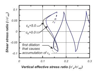
Fig. 3. Effects of input parameter c<sub>b</sub> (fabric damage) on contraction rate.
