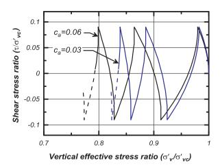
Fig. 2. Effects of input parameter  $c_a$  on contraction rate.
