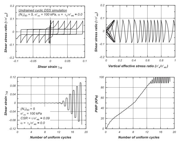
Fig. 9. Example model response in undrained cyclic simple shear loading for  $(N_1)_{60} = 5$ .
