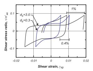
Fig. 7. Effects of input parameter  $d_b$  (fabric damage) on dilation rate.
