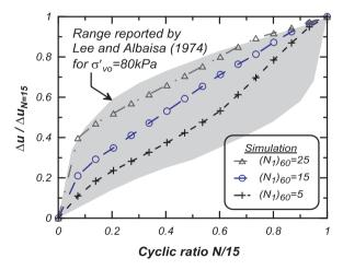
Fig. 10. Model predicted rate of pore pressure generation in DSS simulations for different relative densities at  $\sigma'_{vc}$  = 100 kPa compared with the range expected from experimental observations.
