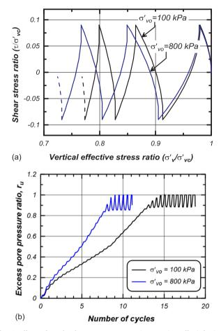
**Fig. 4.** Effects of overburden stress on contraction rate ( $K_{\sigma}$  effect) for input parameter  $c_c = 0.2$ ; (a) stress path and (b) pore water pressure ratio versus number of shear cycles.
