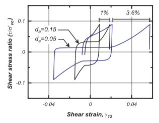
Fig. 6. Effects of input parameter  $d_a$  on dilation rate.
