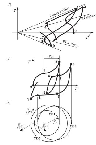
**Fig. 8.** Schematic of the neutral phase in model response showing (a) octahedral stress  $\tau$ - effective confinement p' response, (b)  $\tau$  - octahedral strain  $\gamma$  response, and (c) configuration of yield domain.
