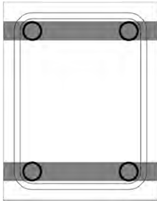
Fig. 3. Cross section of reinforced concrete beam. Reinforced zones containing longitudinal bars shaded.
