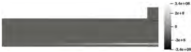
Fig. 7. Axial stresses (N/m 2 ) in longitudinal bars at peak force.
