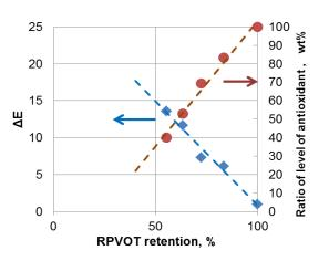
Figure 5. Relationship between RPVOT retention and  $\Delta E$ , and antioxidant ratio as measured in deteriorated EMTO
