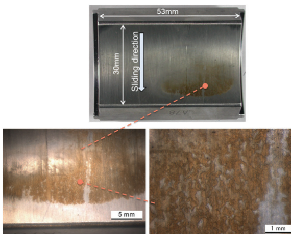
Fig. 1 Example deposit formed on the loaded part of the tilting bearing pad
