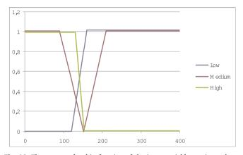
Fig. 10. The non-membership function of the input variable maximum heart rate.
