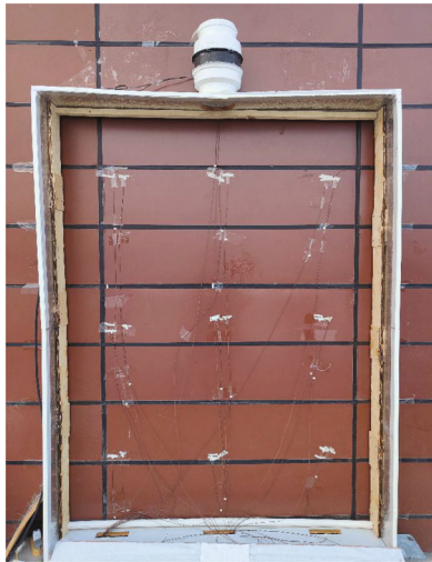
FIGURE 2: Physical diagram of heat recovery type of heat storage wall.
