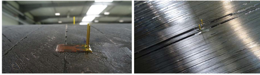
Figure 2. Positioning and embedding of the strain gauge in the middle plane of a CFRP tube.
