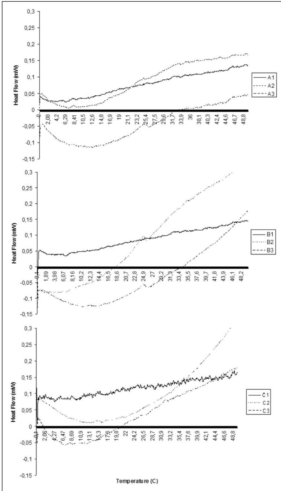
Figure 11. DSC curves of spacer samples.
