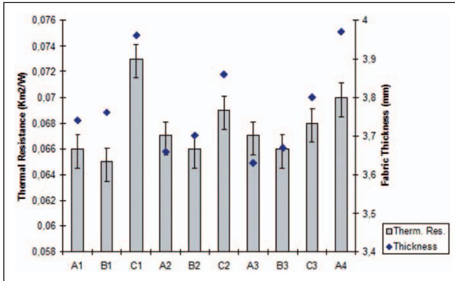
**Figure 7.** The relation of thermal resistance and fabric thickness with the sample codes.
