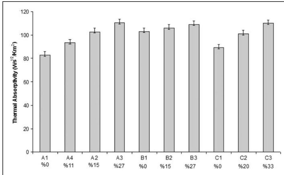
**Figure 8.** Thermal absorptivity values of spacer fabrics versus the Outlast<sup>®</sup> fiber percentage and sample codes.
