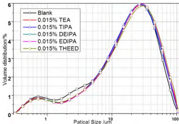
Fig. 4. Particle size distribution of cements powder without and with 0.015% alkanolamines ground for 25 min.
