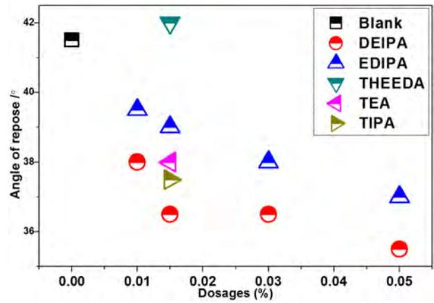
Fig. 5. The angles of repose of cements without and with different alkanolamines ground for 25 min.
