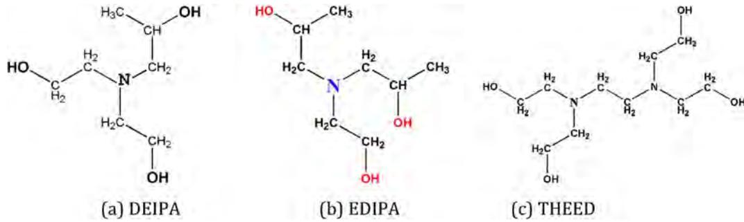
Fig. 1. The molecular structure of DEIPA, EDIPA and THEED.
