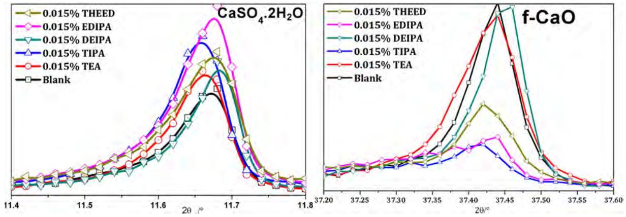
Fig. 9. Contrast of X-ray diffraction peak intensity of samples with alkanolamines ground for 25 min.
