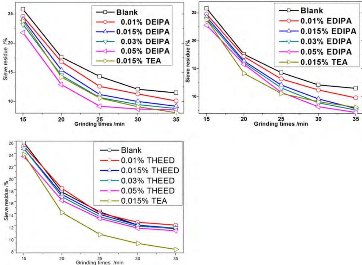
Fig. 2. The sieve residues (45  $\mu\text{m}$ ) of cements powder ground without and with alkanolamines for different times.
