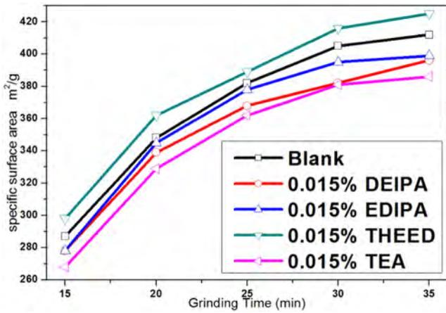
Fig. 3. Blaine specific surface area of cement powder without and with alkanolamines ground for different times.
