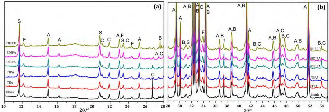
Fig. 8. XRD patterns of samples with different alkanolamines ground for 25 min at the windows of 10–28° 2 $\theta$  (a) and 28–55° 2 $\theta$  (b). The main reflection peaks of C<sub>3</sub>A (C), Ferrite (F), gypsum (S), C<sub>3</sub>S (A), C<sub>2</sub>S (B) and F-CaO (f) are labeled.
