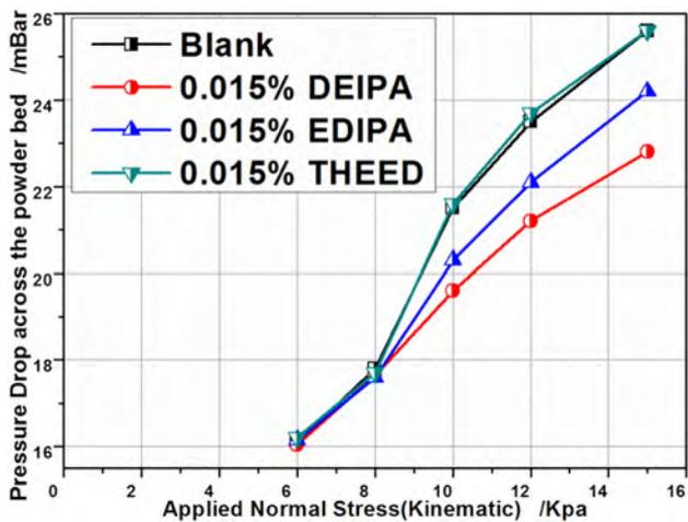
Fig. 7. The values of pressure drop across the powder bed with 2 mm/s air velocity at different applied normal stresses.
