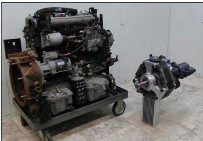
Figure 8. size comparison of a 40hp X engine with a typical naturally aspirated industrial diesel engine Isuzu D201 (35hp)
