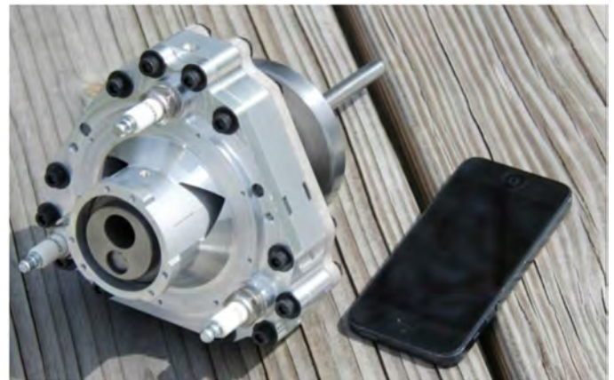
Figure 12. XMv3 engine in comparison to an iPhone for scaling
