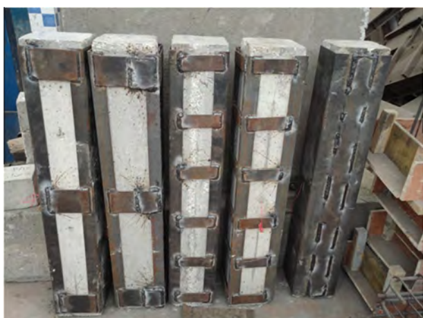
Fig. 2 Strengthened specimens after casting and jacket erection.
