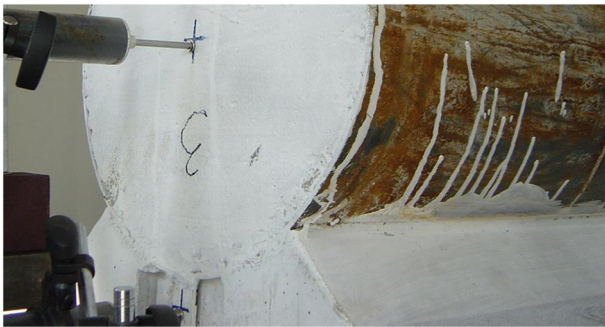
Fig. 14. Slip and cracks at the end of the test specimen (FC-N, Final stage).
