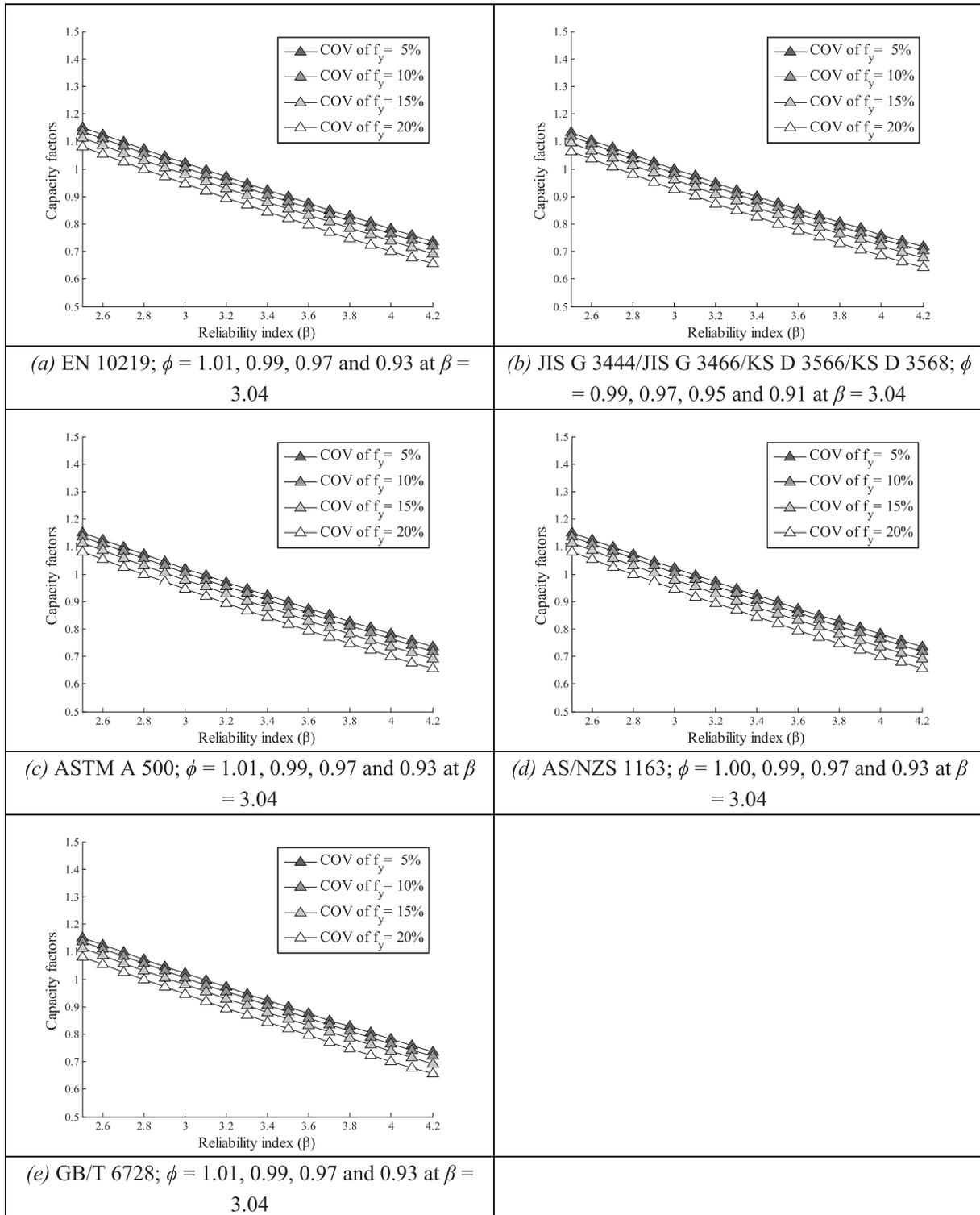
Fig. 12. The capacity factors for steel in rectangular long CFST columns for the various coefficient of variation for the yield strength of steel.
