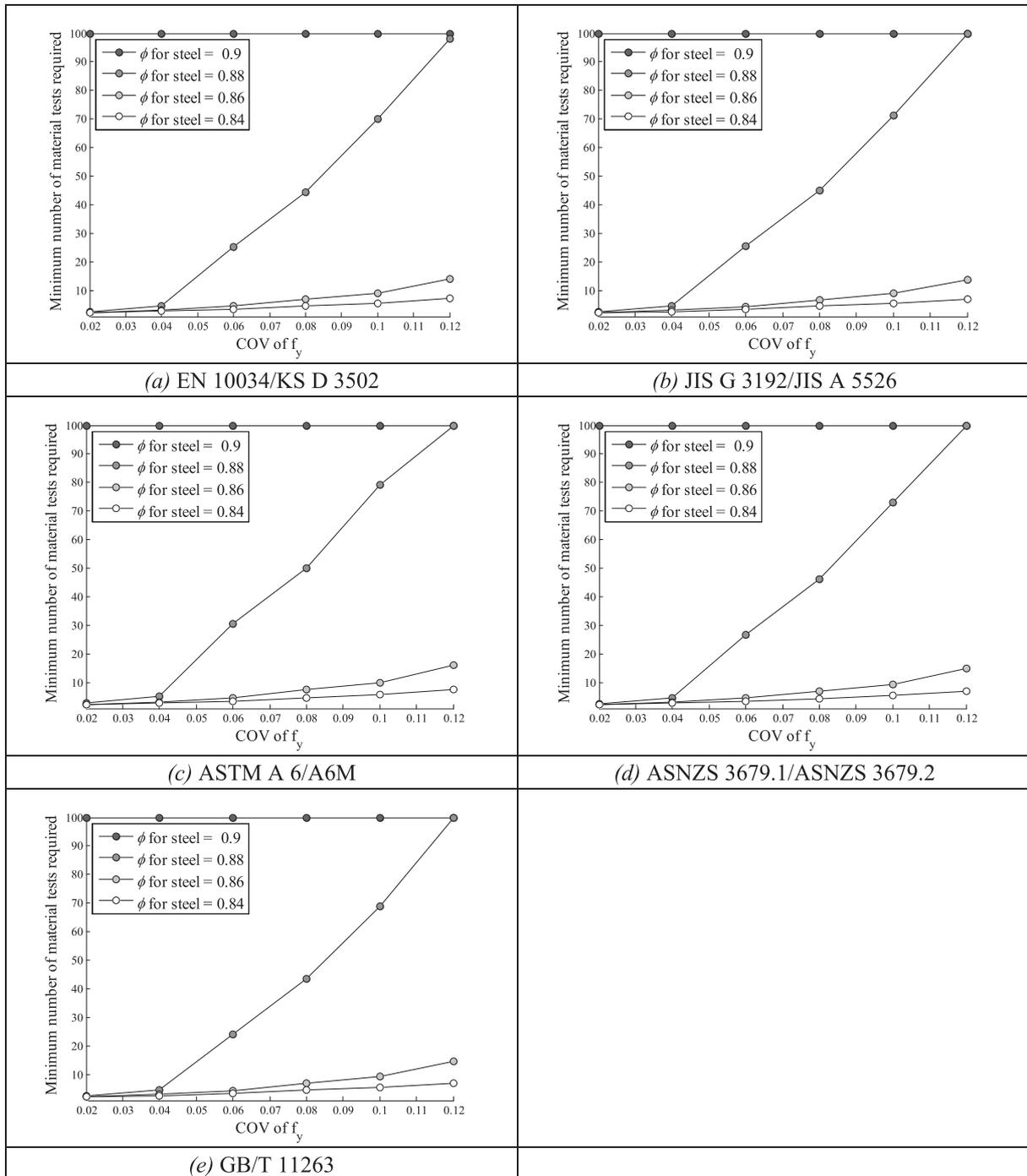
Fig. 20. The required minimum number of yield strength tests for composite beams.
