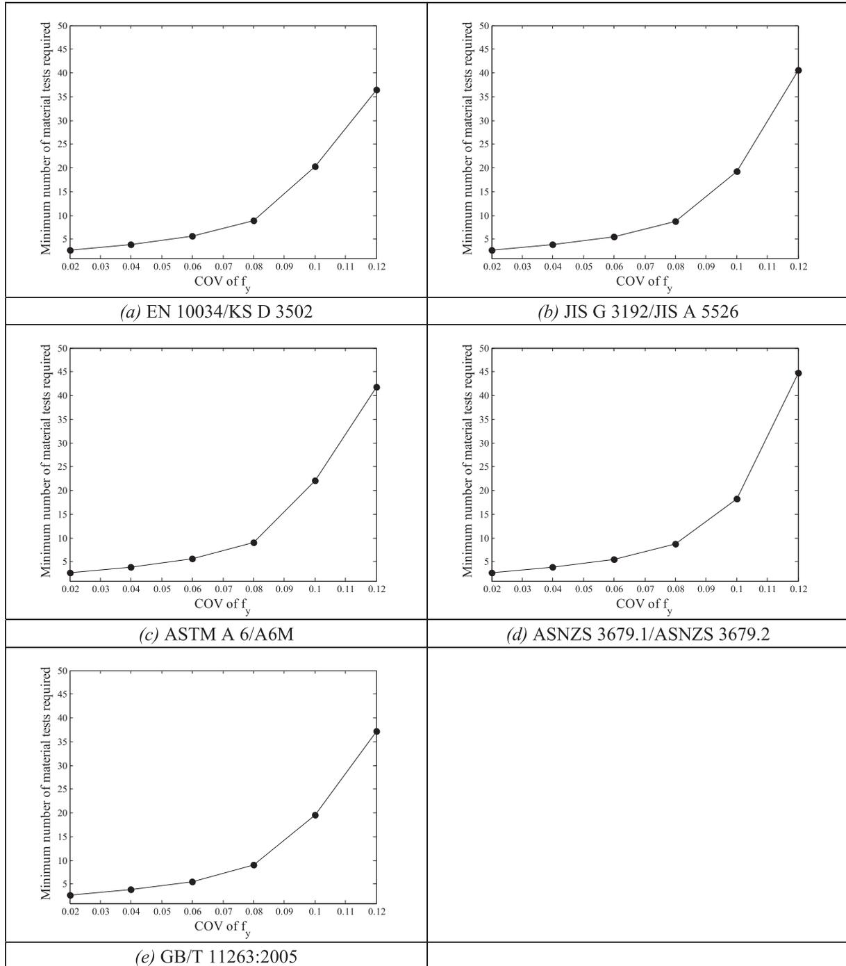
Fig. 6. The minimum number of material tests required to achieve  $\phi = 0.90$  not-compact I sections using products complying with manufacturing tolerances given in international design codes.
