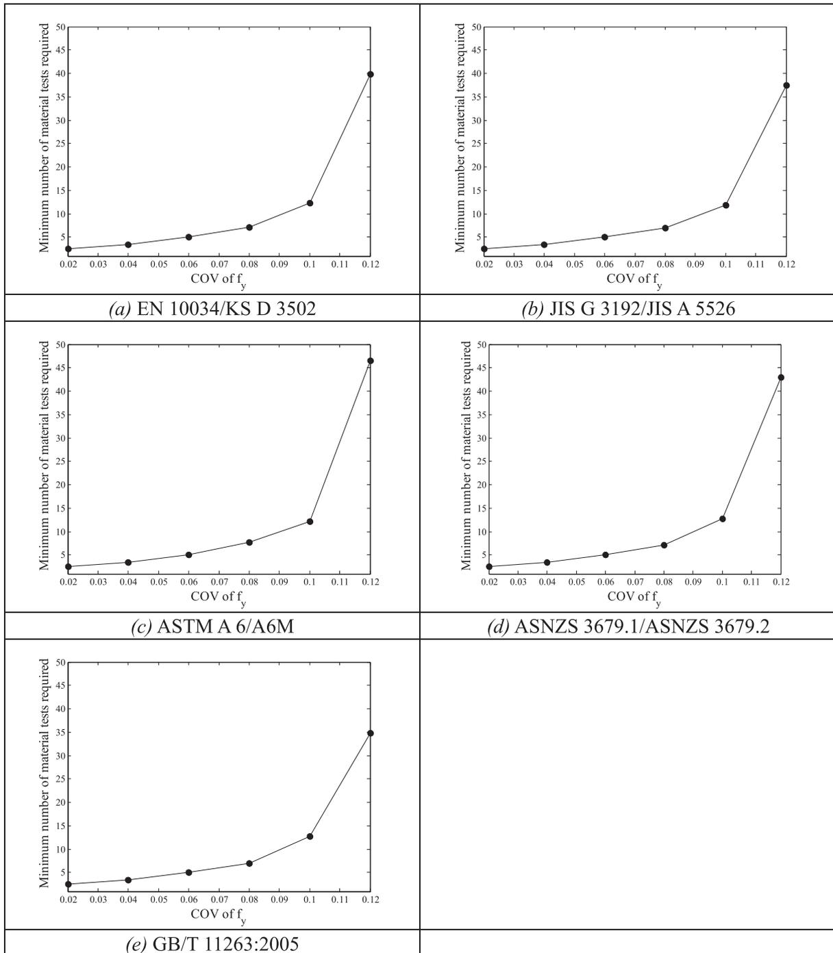
Fig. 7. The minimum number of material tests required to achieve  $\phi = 0.90$  non-compact I sections using products complying with manufacturing tolerances given in international design codes.
