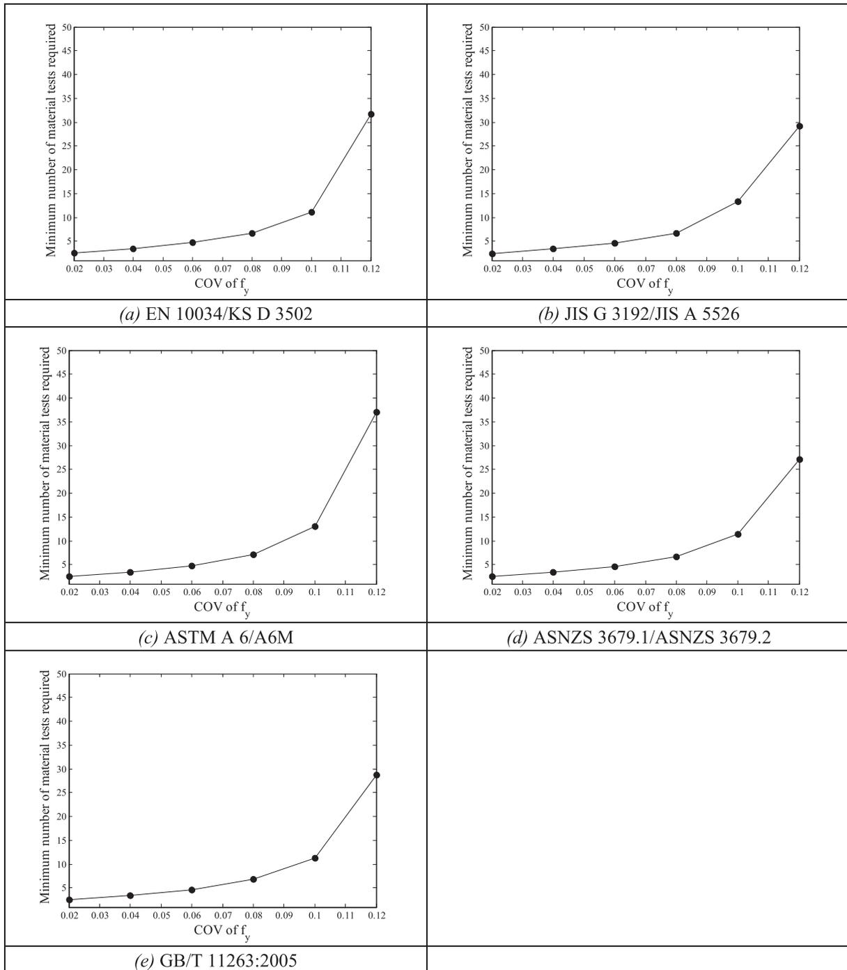
Fig. 5. The minimum number of material tests required to achieve  $\phi = 0.90$  for compact I sections using products complying with manufacturing tolerances given in international design codes.
