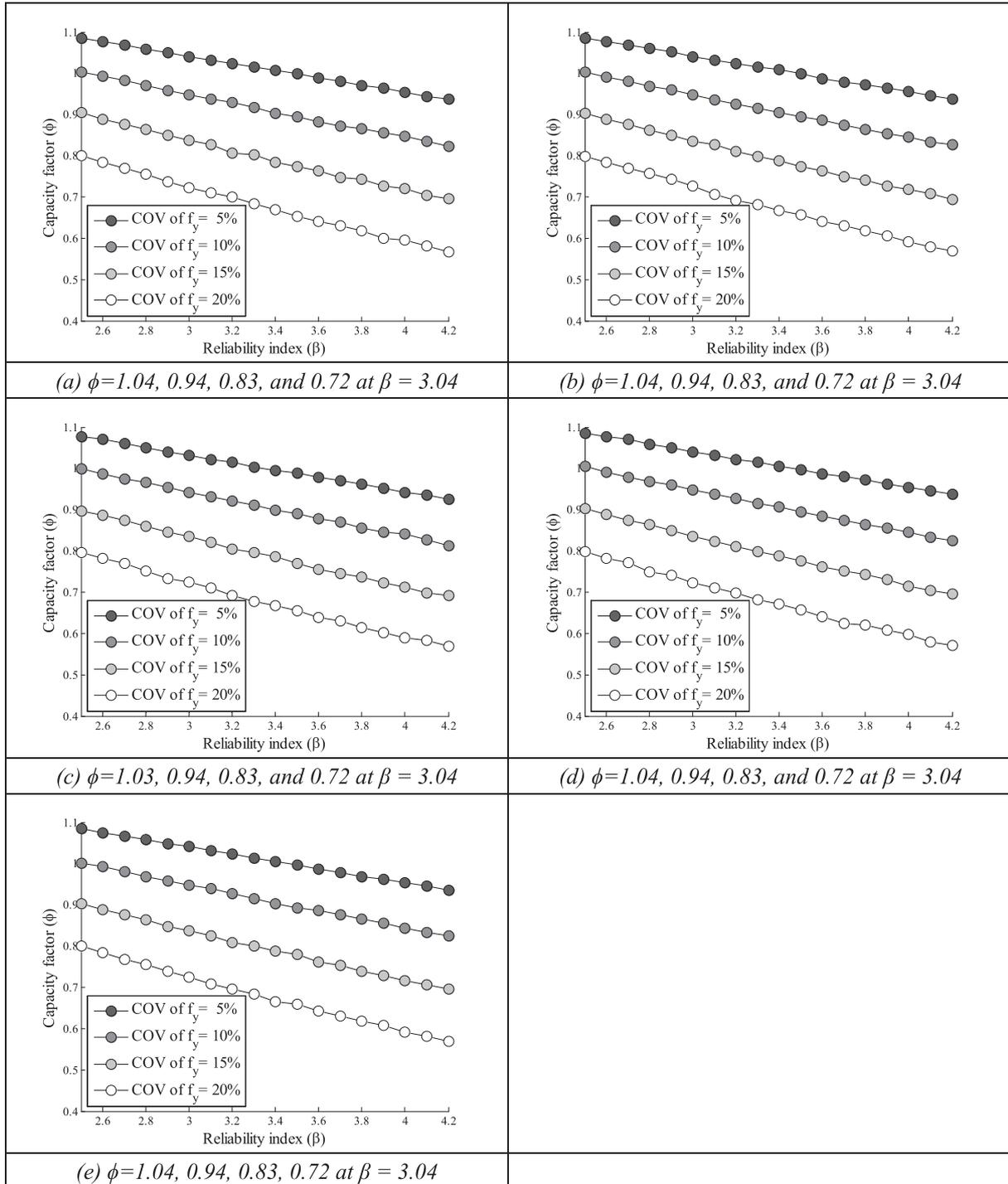
**Fig. 3.** Capacity factors versus reliability index for not-compact I sections using products complying with manufacturing tolerances given in (a) EN 10034/KS D 3502 (b) JIS G 3192/JIS A 5526 (c) ASTM A 6/A6M (d) ASNZS 3679.1-ASNZS 3679.2 (e) GB/T 11263:2005.
