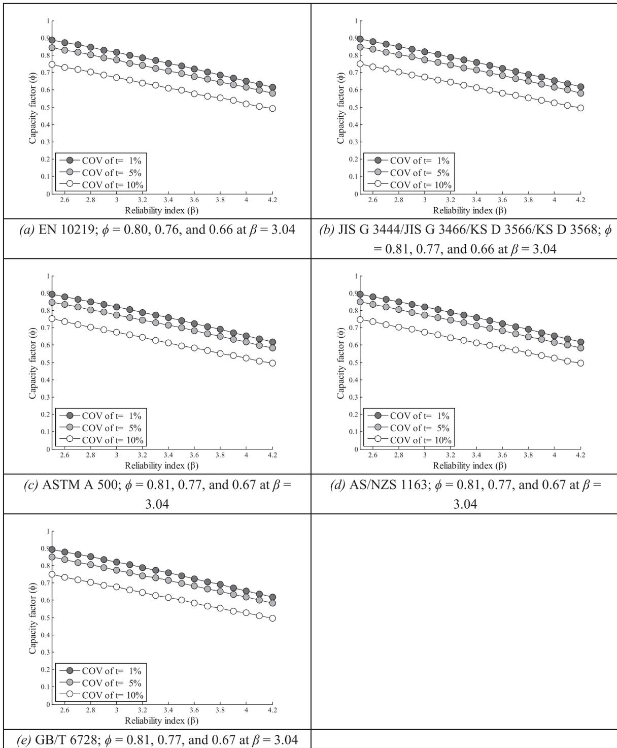
**Fig. 8.** The capacity factors for hollow section columns using products complying with manufacturing tolerances given in international design codes when the coefficient of variation for the yield strength of steel is 10%.
