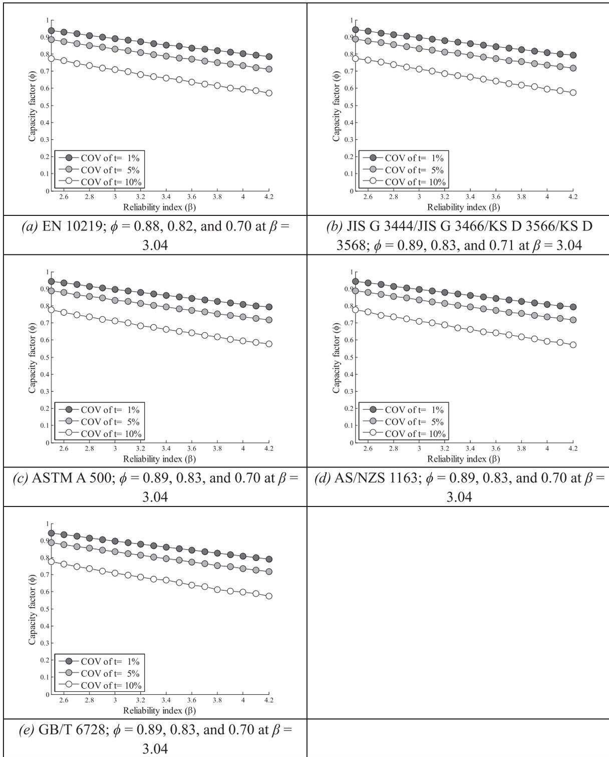
**Fig. 10.** The capacity factors for hollow section columns using products complying with manufacturing tolerances given in international design codes when the coefficient of variation for the yield strength of steel is 7% with the uncertainty due to the insufficient data neglected.
