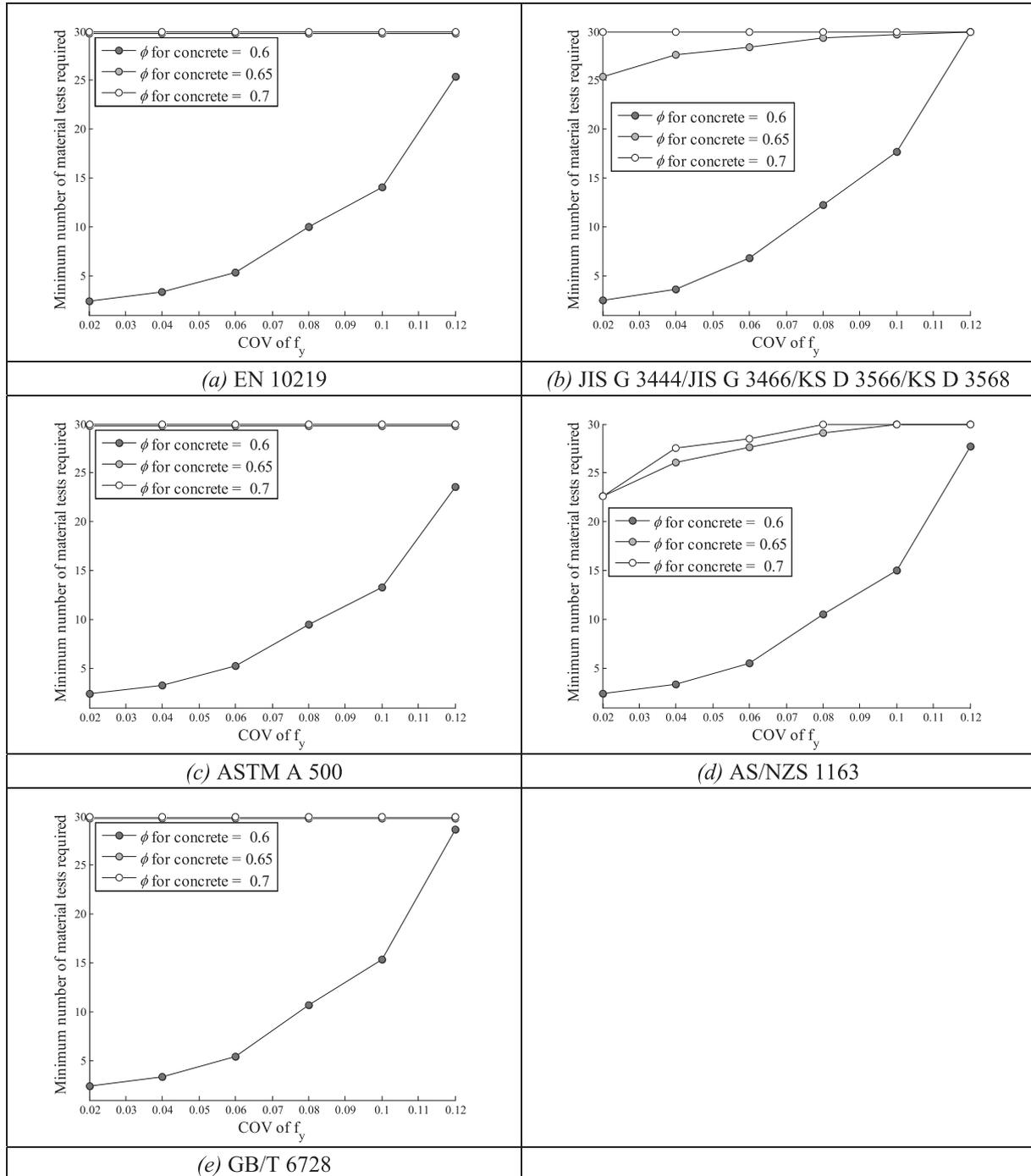
Fig. 17. The required minimum number of yield strength tests for circular stub CFST columns.
