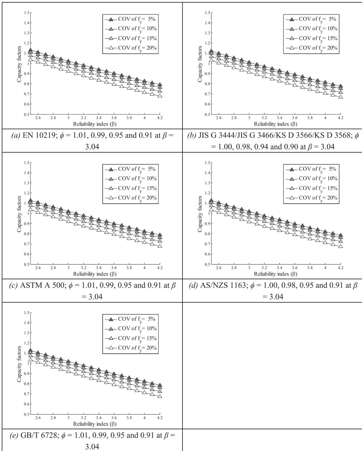
Fig. 14. The capacity factors for steel in circular long CFST columns for the various coefficient of variation for the yield strength of steel.
