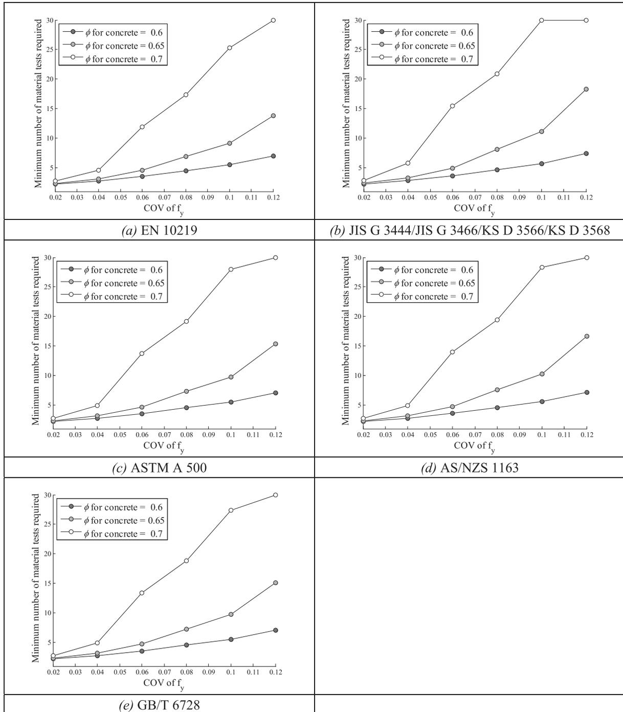
Fig. 15. The required minimum number of yield strength tests for rectangular stub CFST columns.
