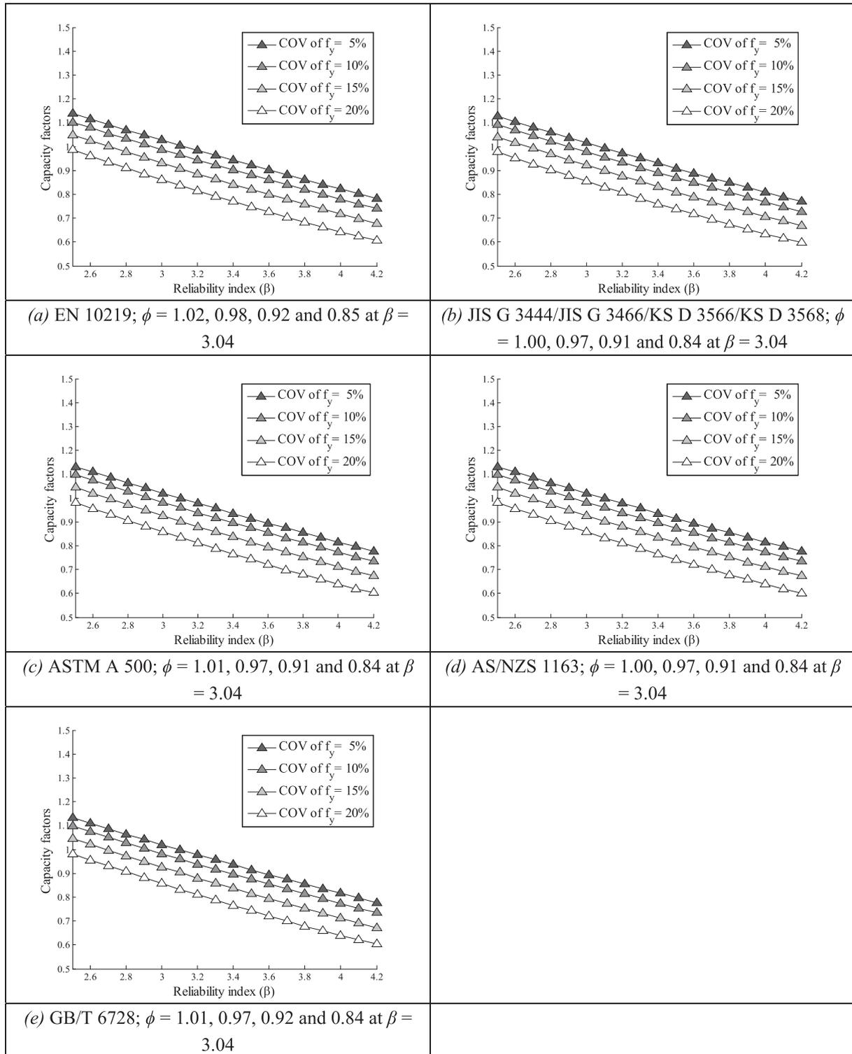
Fig. 11. The capacity factors for steel in rectangular stub CFST columns for the various coefficient of variation for the yield strength of steel.
