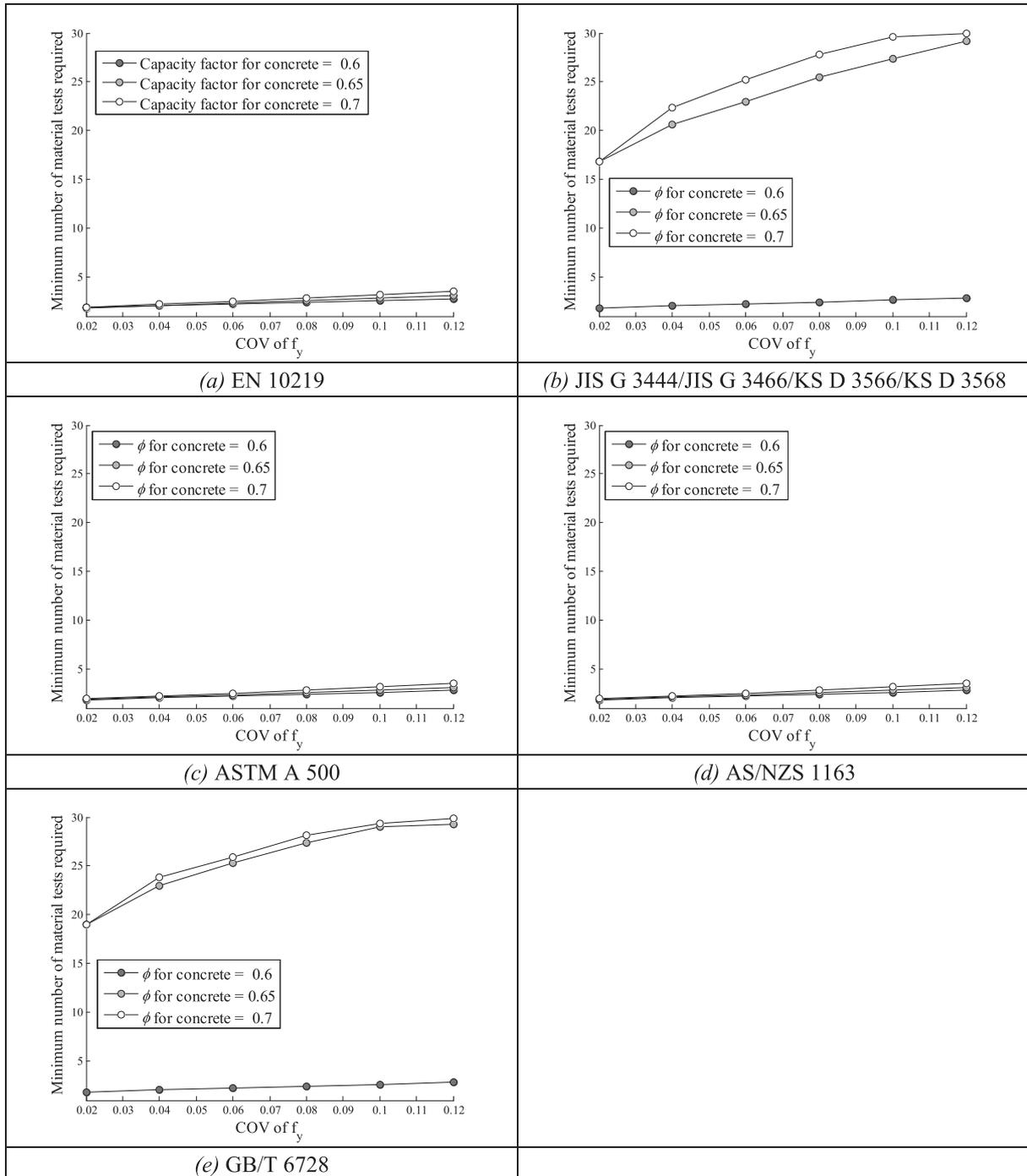
Fig. 16. The required minimum number of yield strength tests for rectangular long CFST columns.
