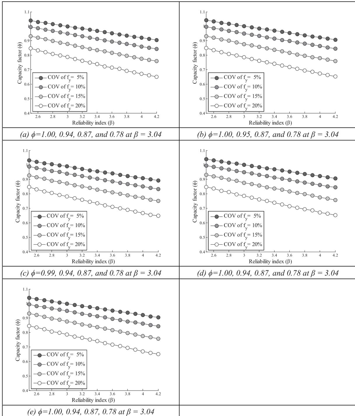
Fig. 2. Capacity factors versus reliability index for compact I sections using products complying with manufacturing tolerances given in (a) EN 10034/KS D 3502 (b) JIS G 3192/JIS A 5526 (c) ASTM A 6/A6M (d) ASNZS 3679.1-ASNZS 3679.2 (e) GB/T 11263:2005.
