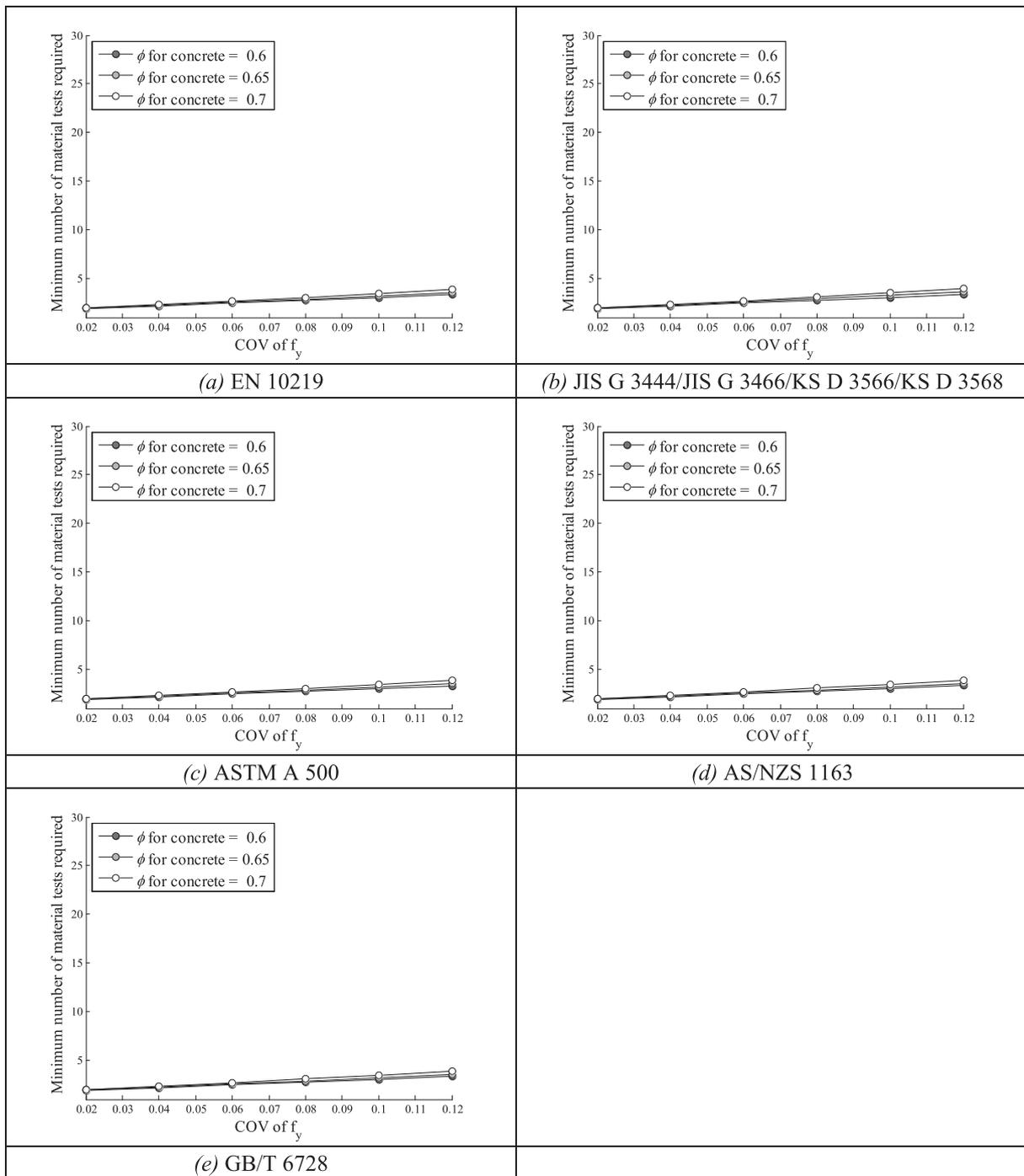
Fig. 18. The required minimum number of yield strength tests for circular long CFST columns.
