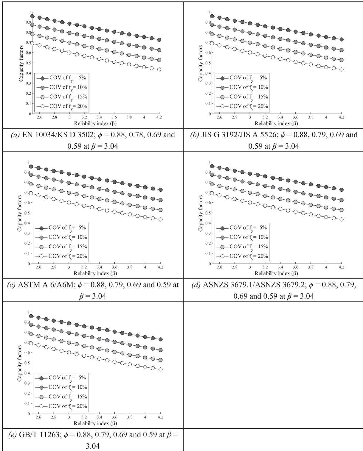
Fig. 19. The capacity factors for steel in composite beams for the various coefficient of variation for the yield strength of steel.
