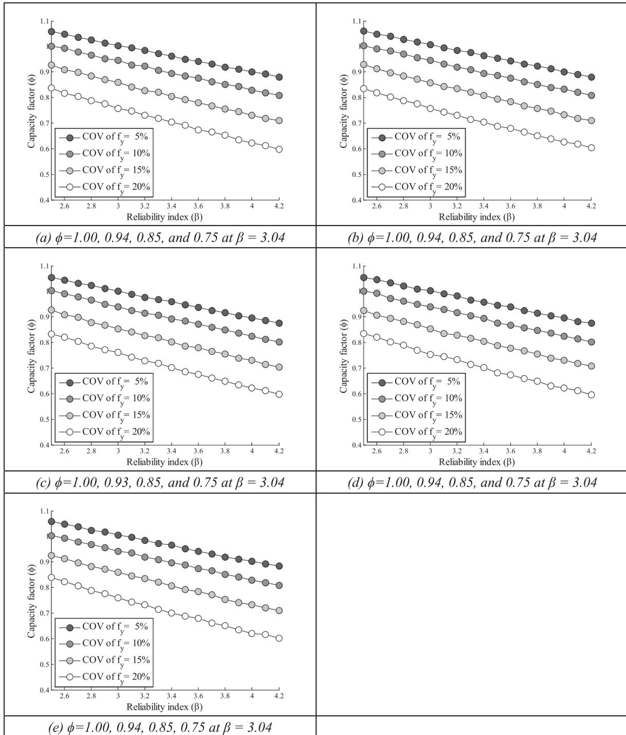
Fig. 4. Capacity factors versus reliability index for non-compact I sections using products complying with manufacturing tolerances given in (a) EN 10034/KS D 3502 (b) JIS G 3192/JIS A 5526 (c) ASTM A 6/A6M (d) AS/NZS 3679.1/AS/NZS 3679.2 (e) GB/T 11263:2005.
