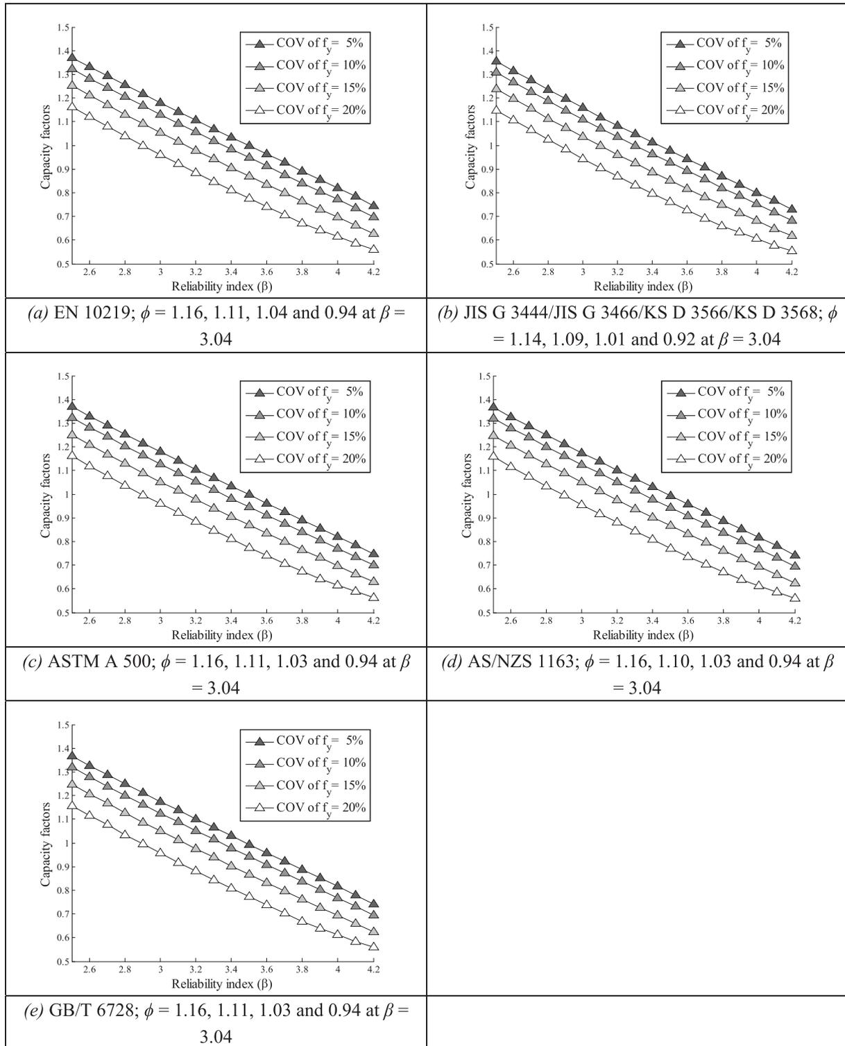
Fig. 13. The capacity factors for steel in circular stub CFST columns for the various coefficient of variation for the yield strength of steel.
