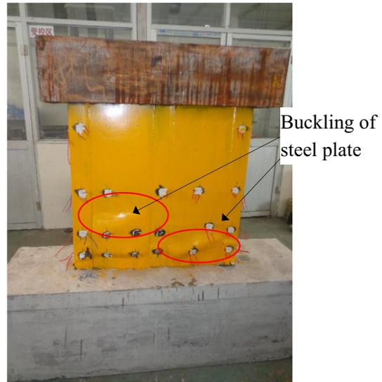
(b) Failure mode II for CWS4
