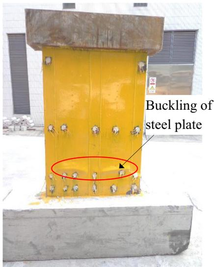
(a) Failure mode I for CWS1
