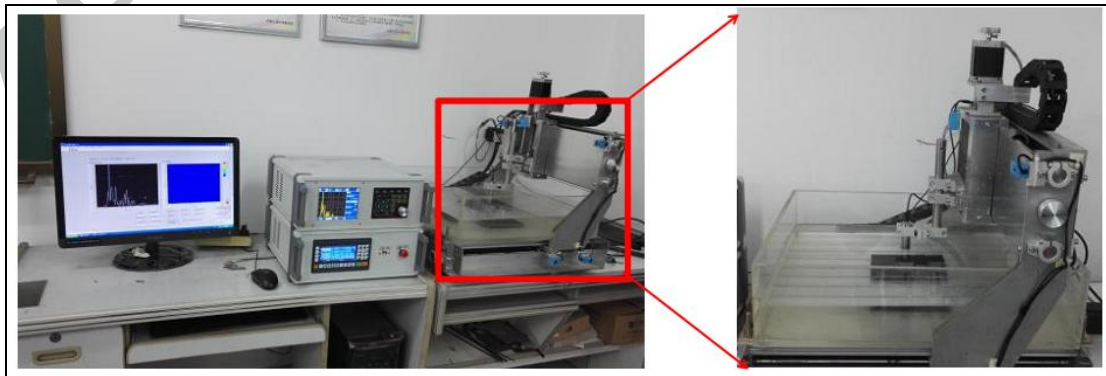
Fig. 3. Immersion focused ultrasound setup
