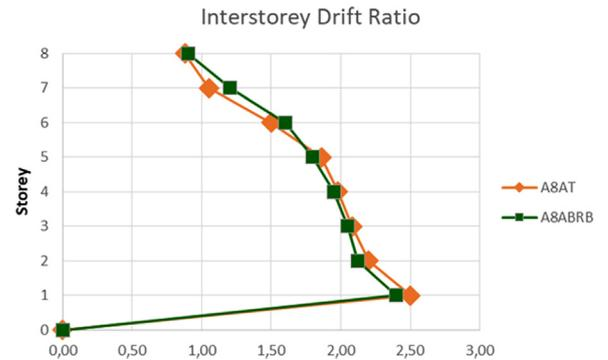
Fig. 11. - Mean peak IDRs for A8a structures.
