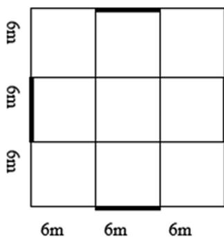
Fig. 2. - Floor plan of Type A structures and location of the braces.
