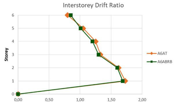
Fig. 10. - Mean peak IDRs for A6a structures.
