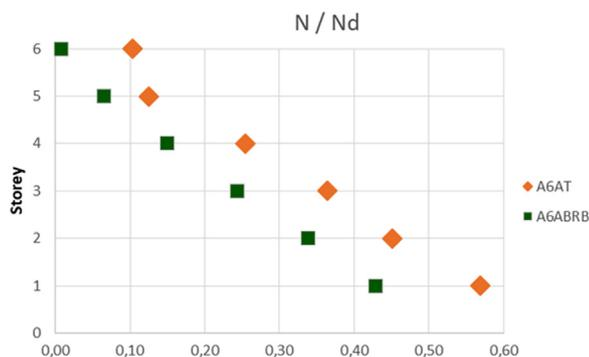
Fig. 22. – Column seismic demands in terms of  $N/N_d$  for A6a structures.
