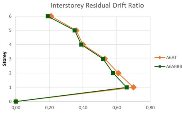
Fig. 14. – Mean peak RIDRs for A6a structures.
