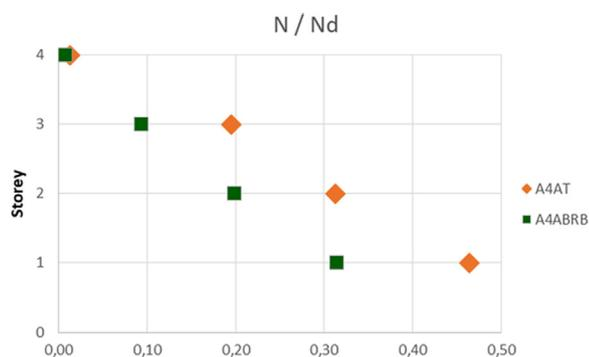
Fig. 21. – Column seismic demands in terms of  $N/N_d$  for A4a structures.
