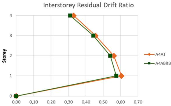
Fig. 13. – Mean peak RIDRs for A4a structures.
