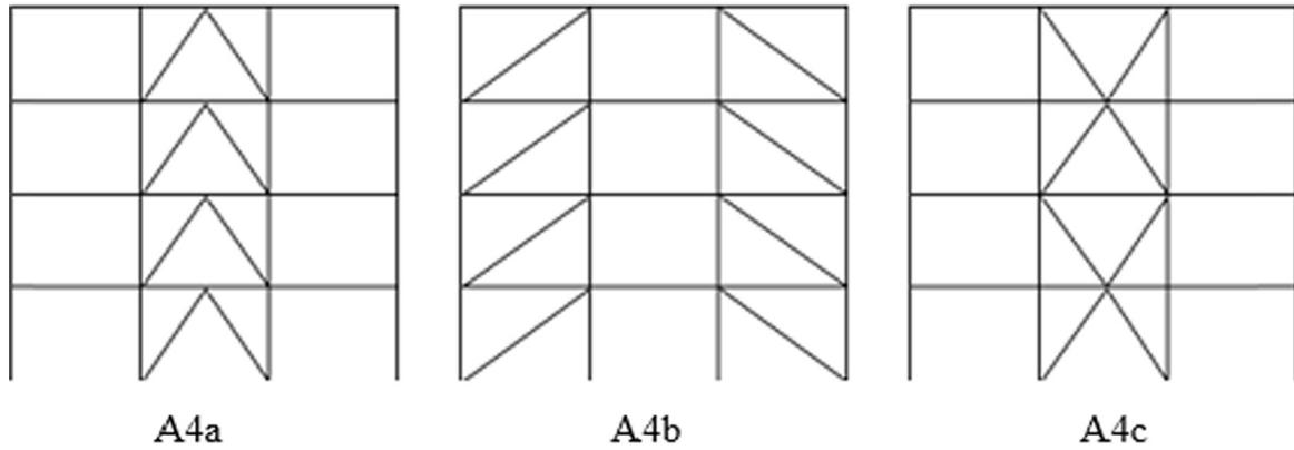
Fig. 4. - Configuration of braces for Type A structures.
