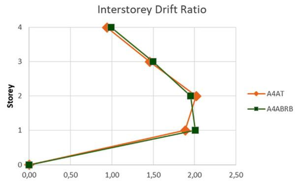
Fig. 9. - Mean peak IDRs for A4a structures.
