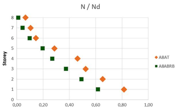
Fig. 23. – Column seismic demands in terms of  $N/N_d$  for A8a structures.
