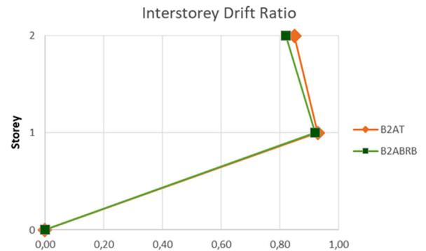
Fig. 12. - Mean peak IDRs for B2a structures.
