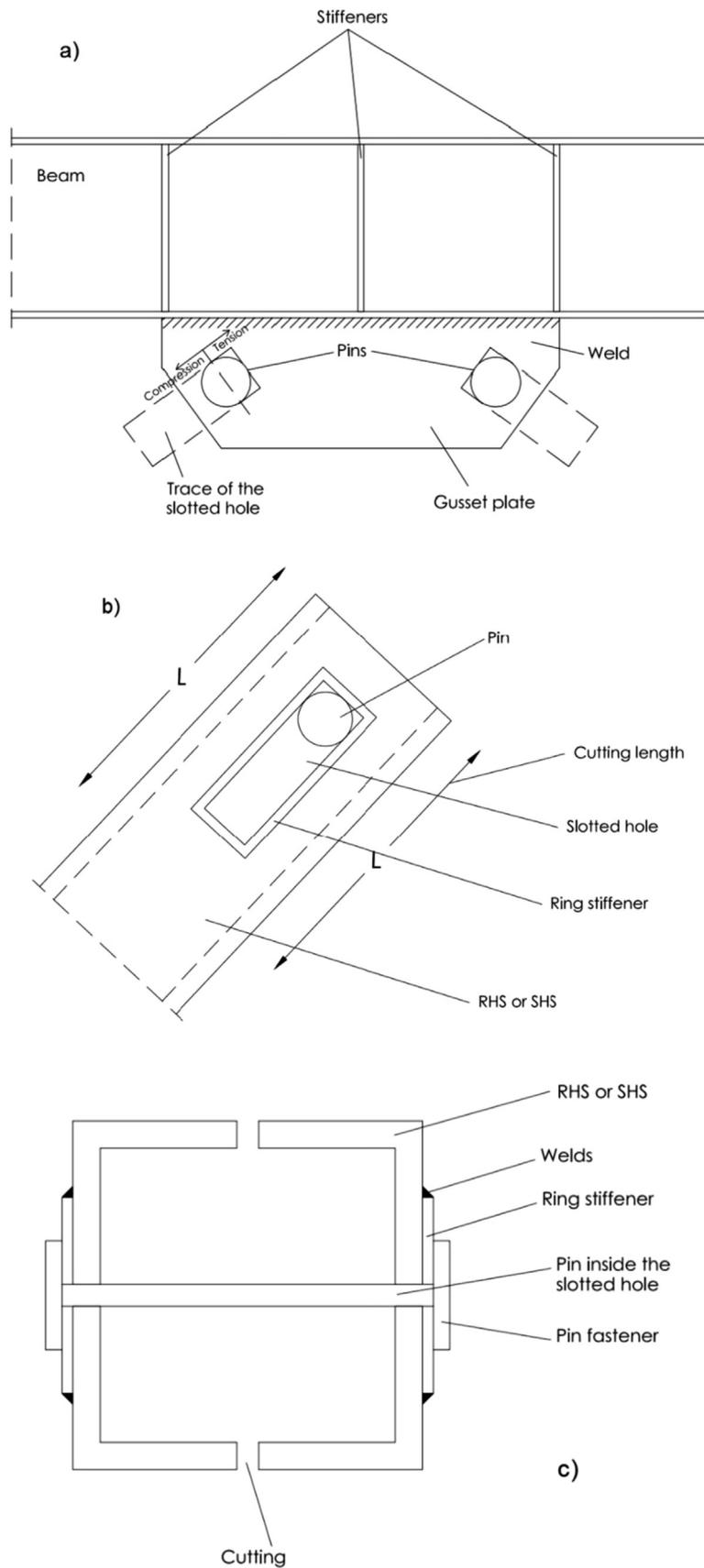
Fig. 1. - Detail of the proposed sliding joint that creates a tension-only brace.
