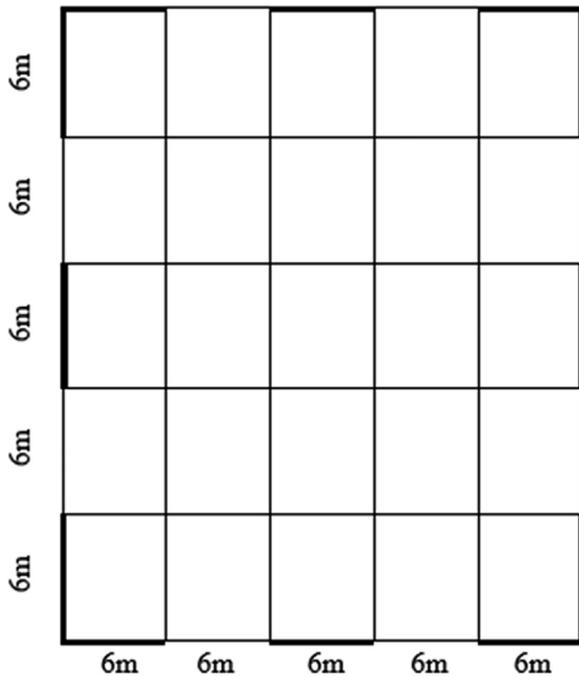
Fig. 5. - Floor plan of Type B structure and location of the braces.
