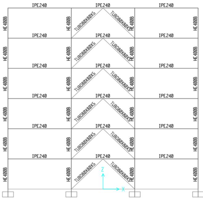
Fig. 7. - Sections at an exterior frame for the A6a structure with tension-only braces.
