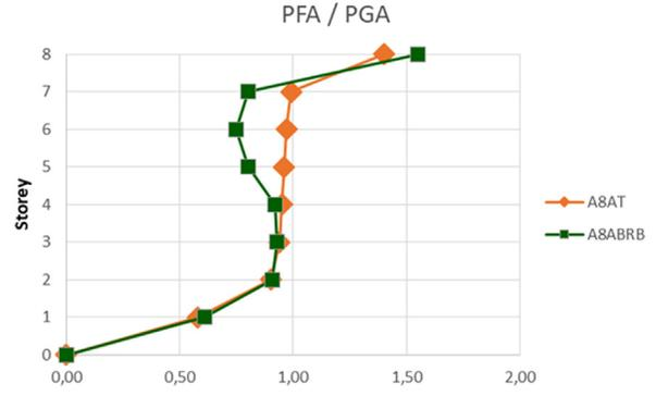
Fig. 19. – Mean peak PFAs for A8a structures.
