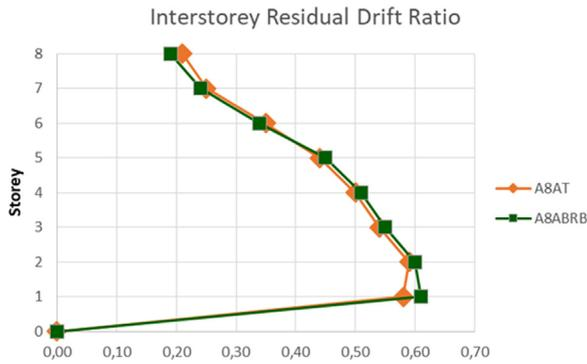
Fig. 15. – Mean peak RIDRs for A8a structures.
