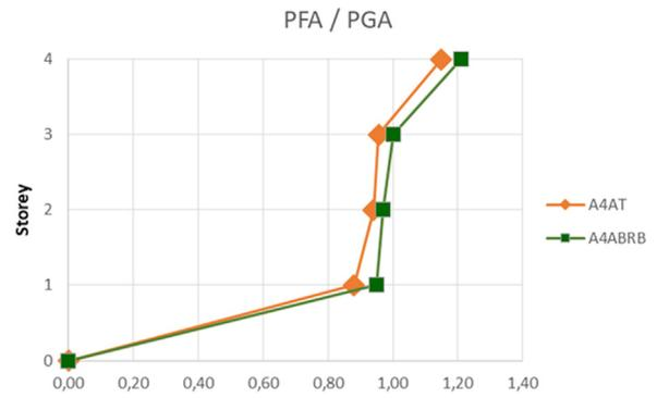
Fig. 17. – Mean peak PFAs for A4a structures.
