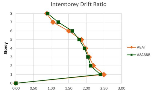
Fig. 11. - Mean peak IDRs for A8a structures.
