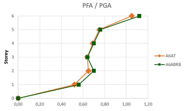
Fig. 18. – Mean peak PFAs for A6a structures.
