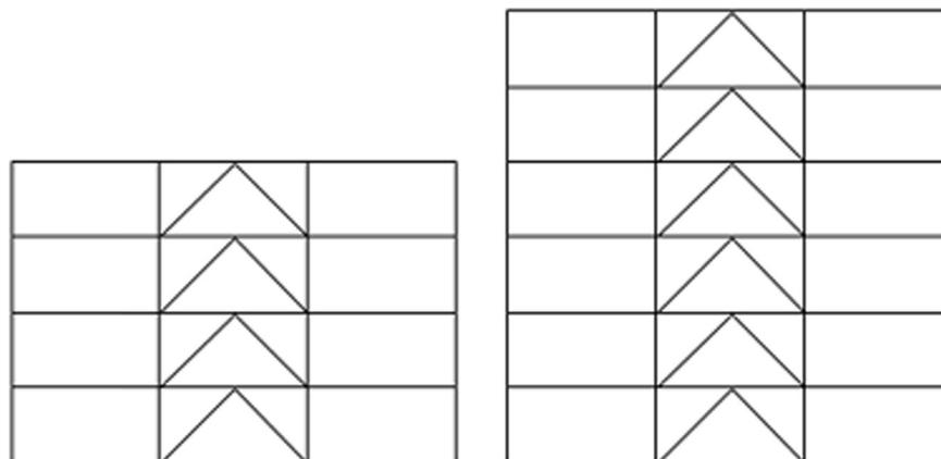
Fig. 3. - Front views of 4- and 6-storey Type A structures.
