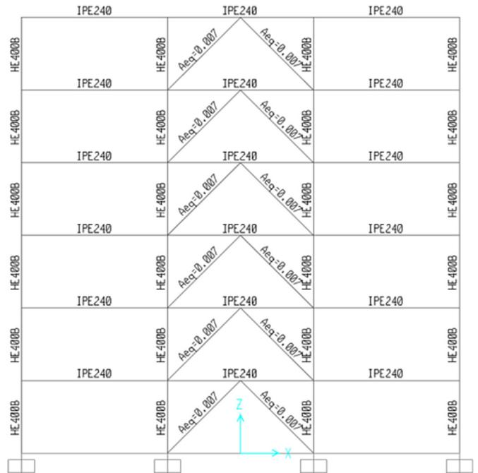
Fig. 6. - Sections at an exterior frame for the A6a structure with BRBs.
