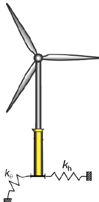
Fig. 7. Schematics of foundation springs or macro-elements in OWTs.
