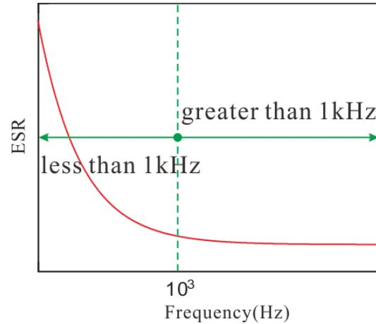
Fig. 3 Typical capacitor ESR frequency characteristic curve.
