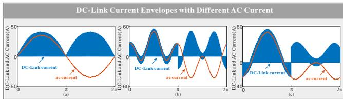
Fig. 5 The dc-link current waveforms at  $M_1=0.8$  when the ac current contains harmonics of: (a)  $I_1=35\text{A}$ ,  $\varphi_1=0$ ; (b)  $I_1=I_2=25\text{A}$ ,  $\varphi_1=\varphi_2=0$ ; (c)  $I_1=I_4=25$ ,  $\varphi_1=\varphi_4=0$ .
