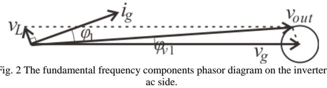
Fig. 2 The fundamental frequency components phasor diagram on the inverter ac side.
