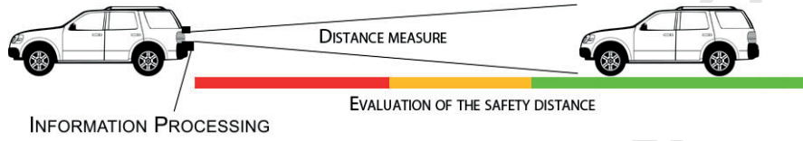
Figure 1: Cooperative driving in which visual data related to the safety distance is provided to the following vehicle in real-time.
