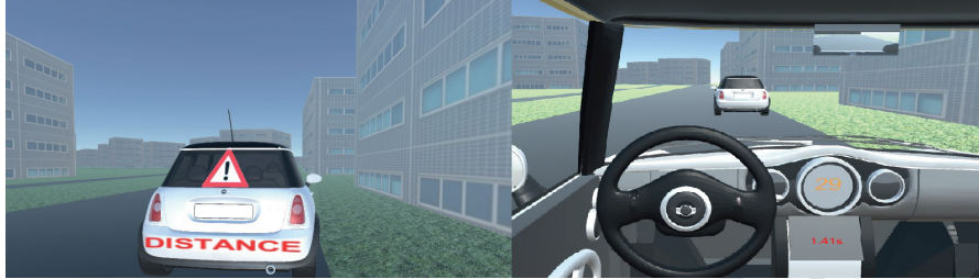
Figure 13: Evaluated systems in the simulation platform. Left: Tailigator rear-end-collision system; Right: VANET system showing the warning on the in-vehicle display and which broadcasts the information related to the headway to the leading vehicle as time gap between vehicles.
