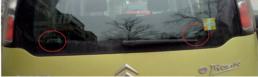
Figure 3: Location of the cameras in the rear part of the vehicle.
