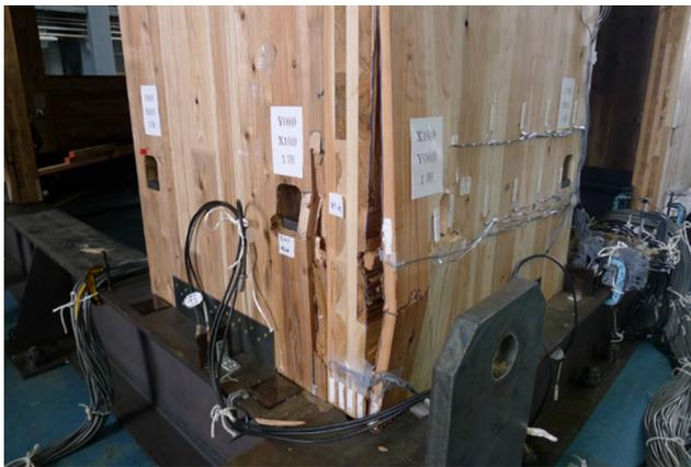
**Fig. 13.** Damage observed during JMA Kobe.
