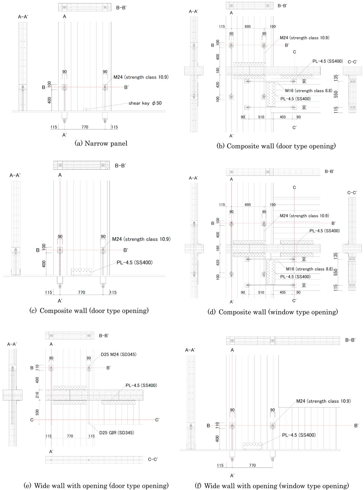
Fig. 2. Connection details [mm].
