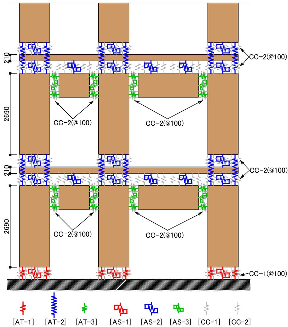
Fig. 9. Numerical model of target structure.
