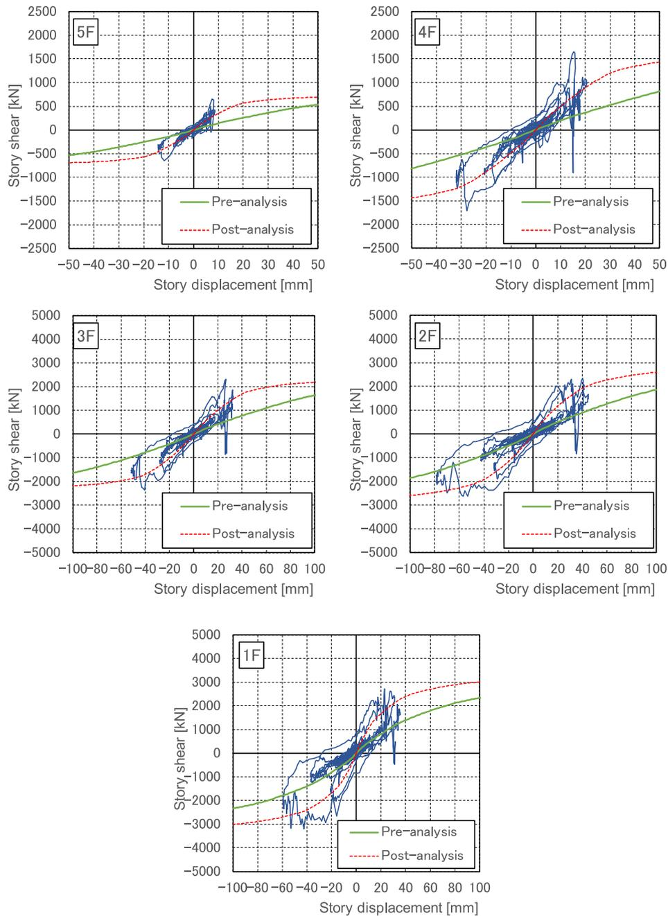
Fig. 14. Comparison between test and analytical results.
