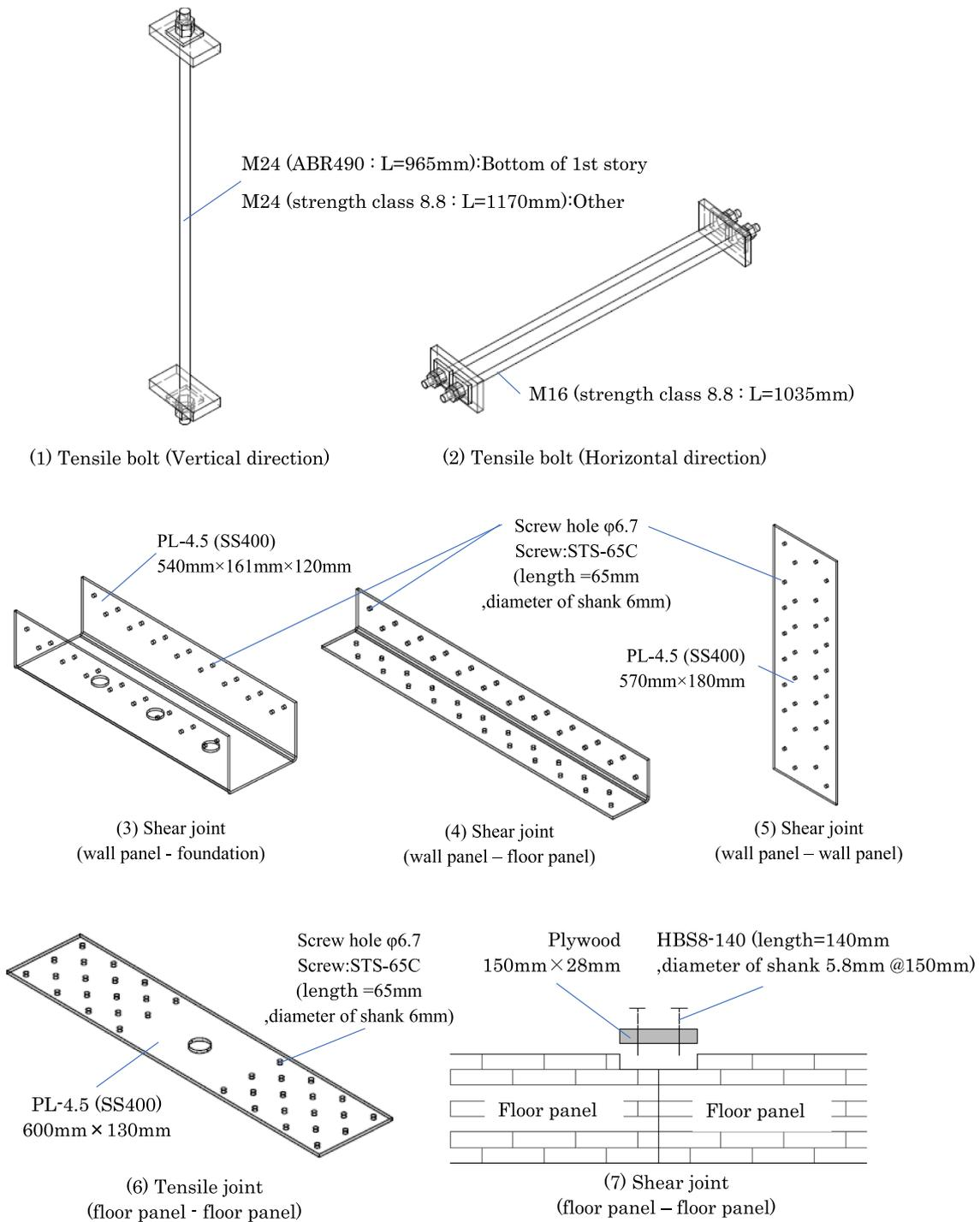
Fig. 7. Detail of connections.
