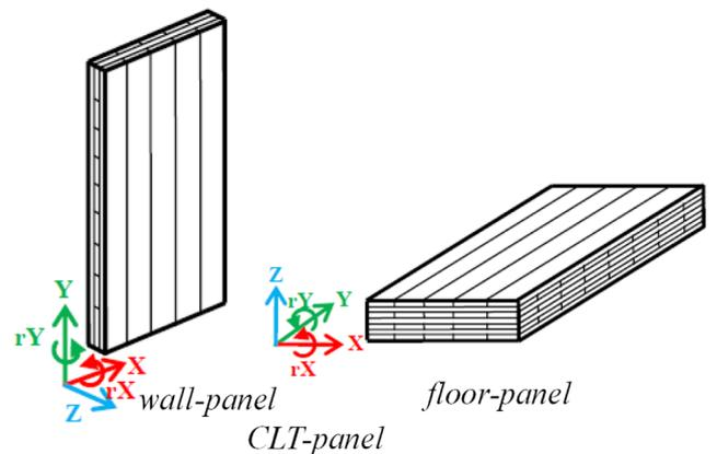
Fig. 10. Definition of direction of CLT panel.
