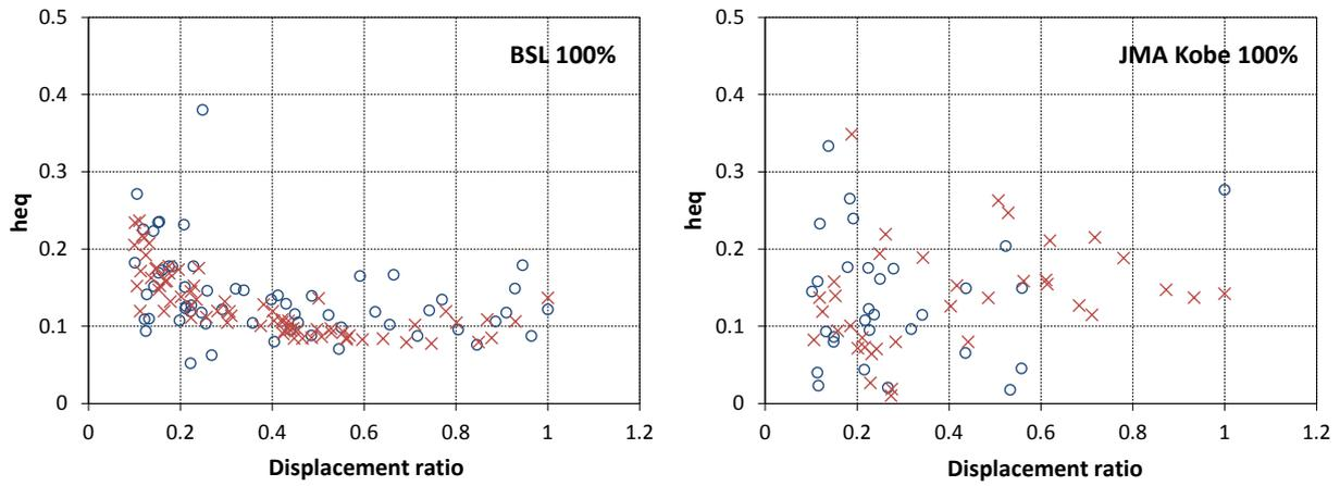
Fig. 15. Equivalent damping ratio from the shaking table test.
