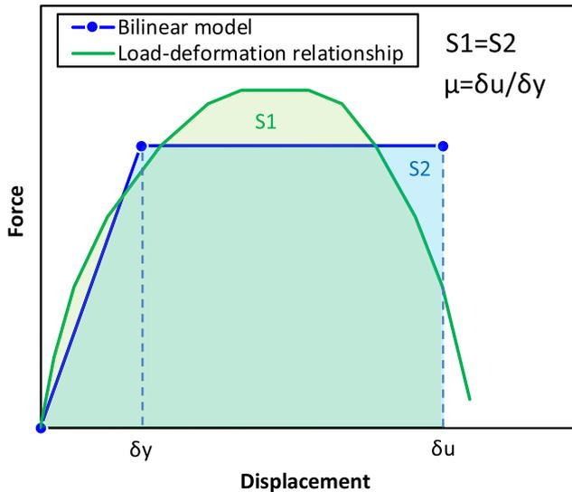
Fig. 3. Definition of ultimate and yield displacement.
