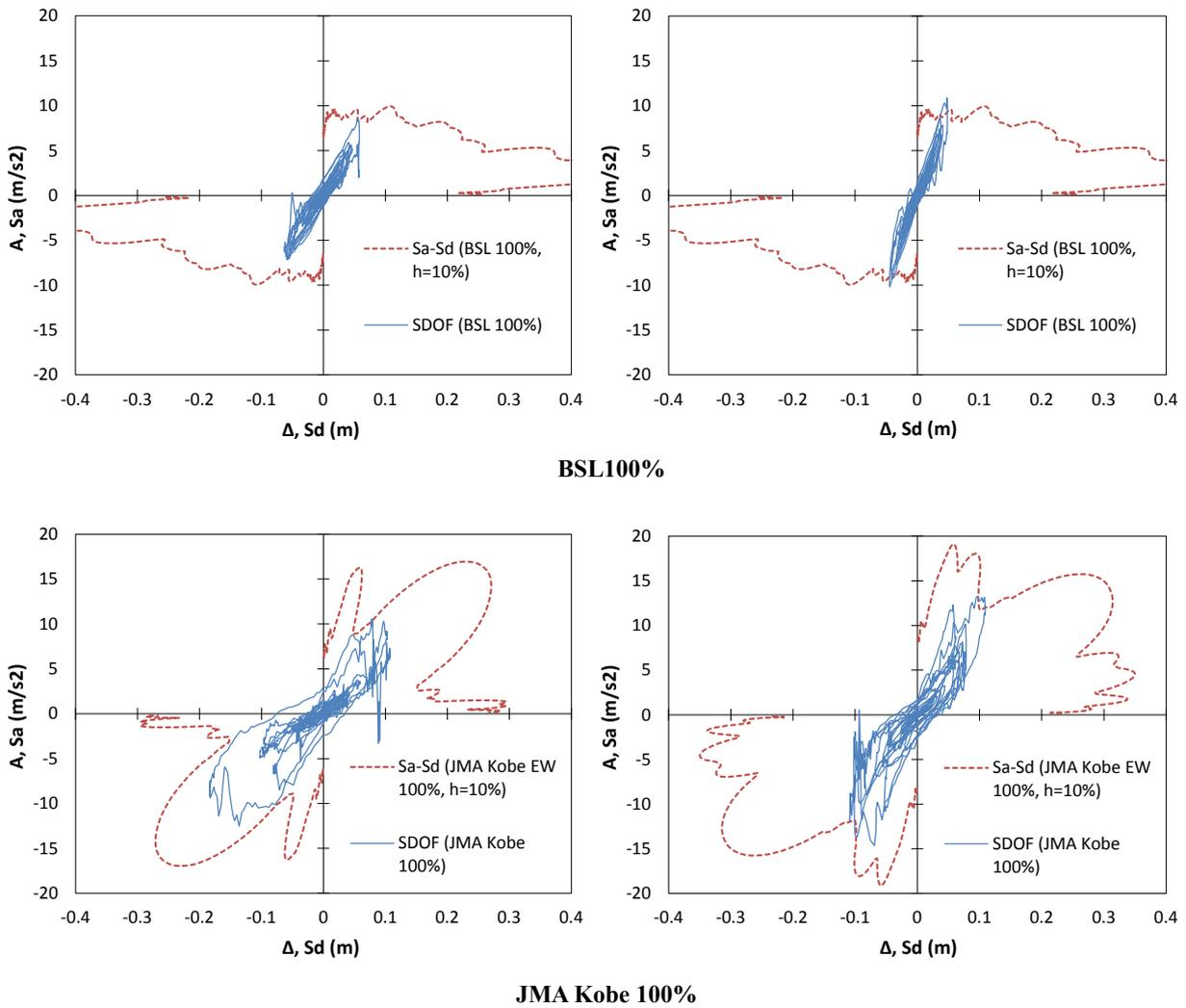
Fig. 16. Relationship between the Sa-Sd spectrum and capacity curve of the SDOF system.
