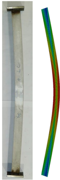
Fig. 11. Experimental and numerical failure modes for beam-column specimen 50Min4 under compression and bending about the minor axis.
