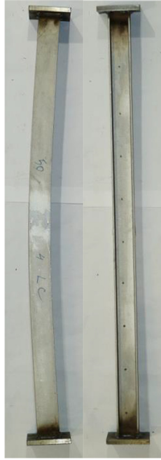
Fig. 6. Typical failure mode for beam-column under combined axial compression and bending about the minor axis (50Min4).
