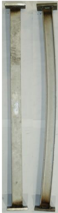
Fig. 10. Typical failure mode for beam-column under combined axial compression and bending about the major axis (50Maj5).
