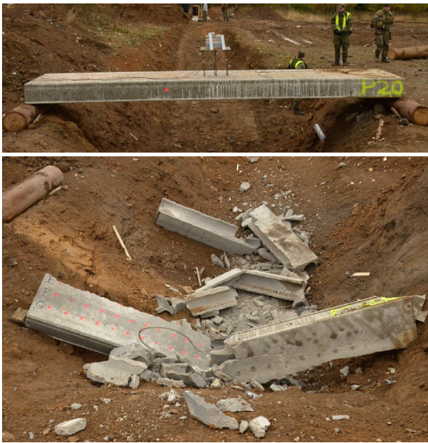
Fig. 8. Specimen No. 20, before (top) and after the blast (bottom).
