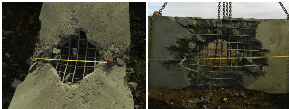
Fig. 5. Damage to reference specimen No. 1 after the blast. Top view (left), bottom view (right).
