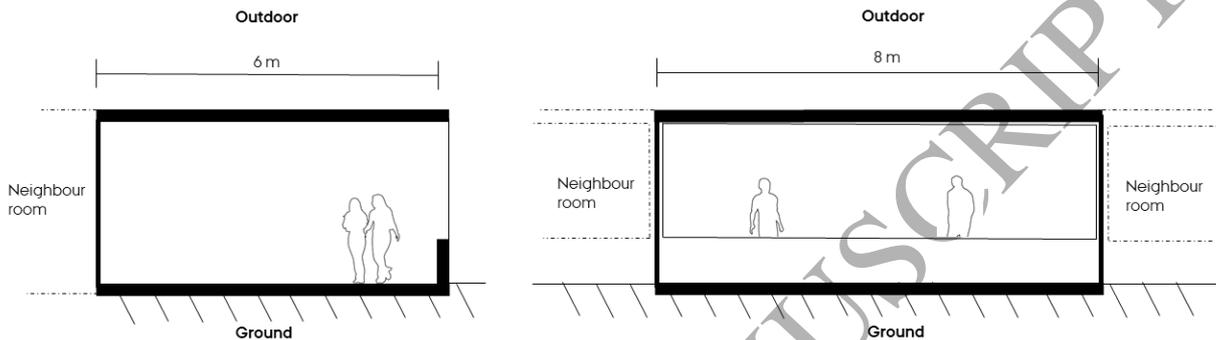
Figure 1. Internal dimensions and boundary conditions for the office building zone. Left: Vertical section of the zone. Right: Front elevation of the façade. The walls facing neighbour rooms are assumed adiabatic.
